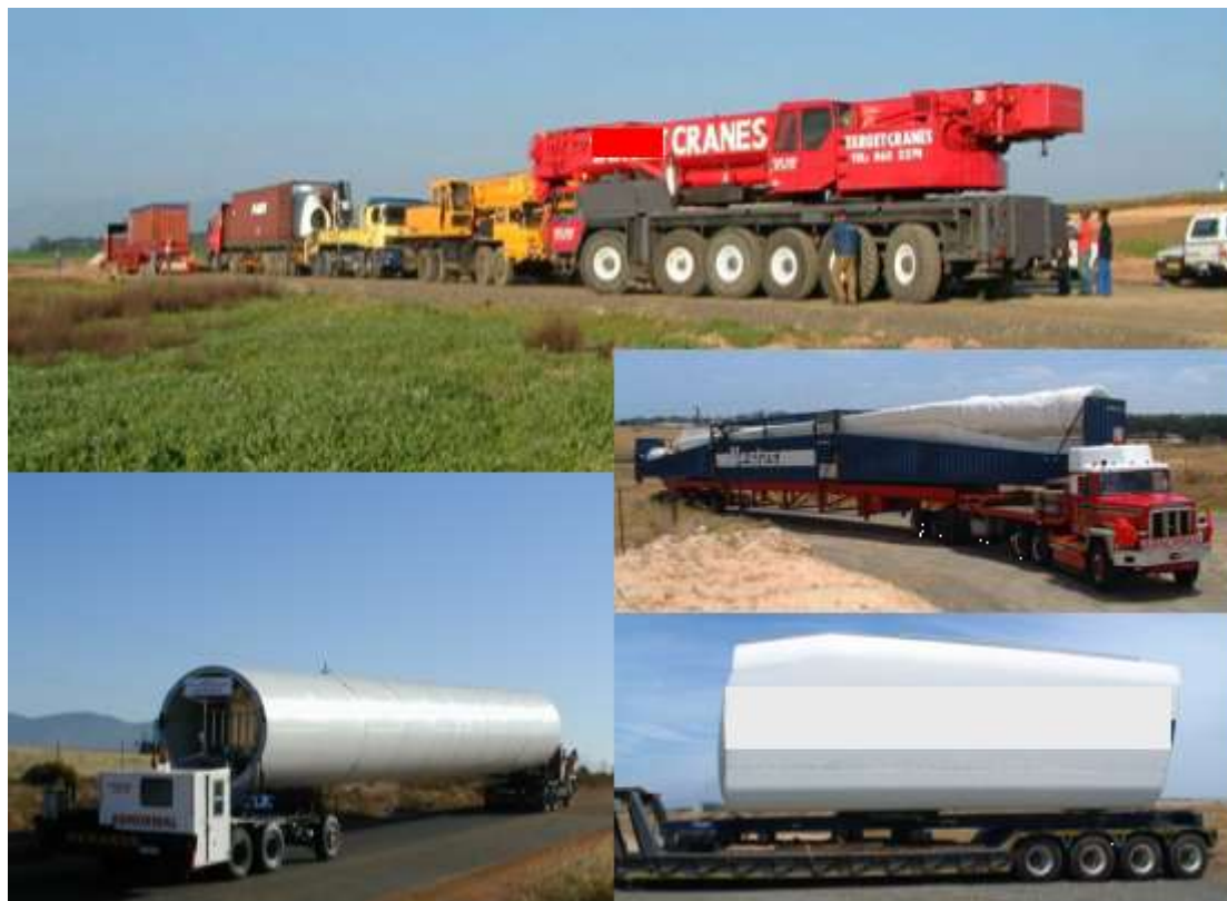
Figure 4.5: Photographs illustrating the equipment required for the transportation of turbine components to site (photographs courtesy of Eskom at during the construction of the Klipheuwel demonstration facility)
