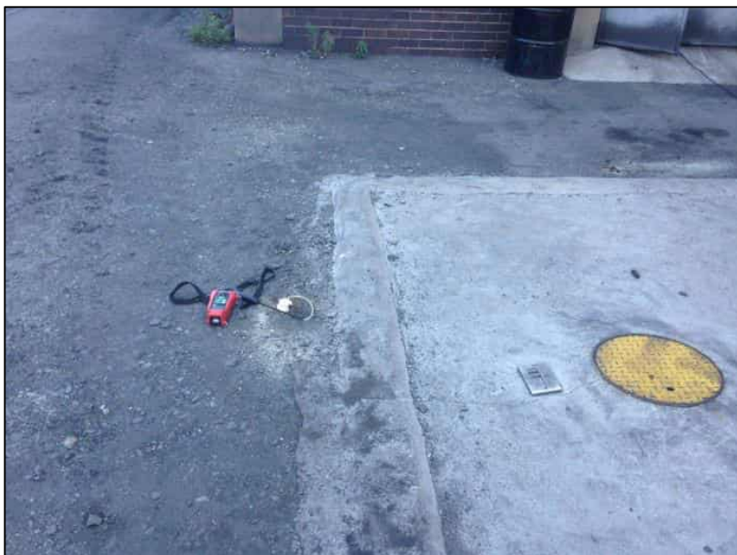
Figure 39: Position of PID measurement (along concrete of diesel storage area)
