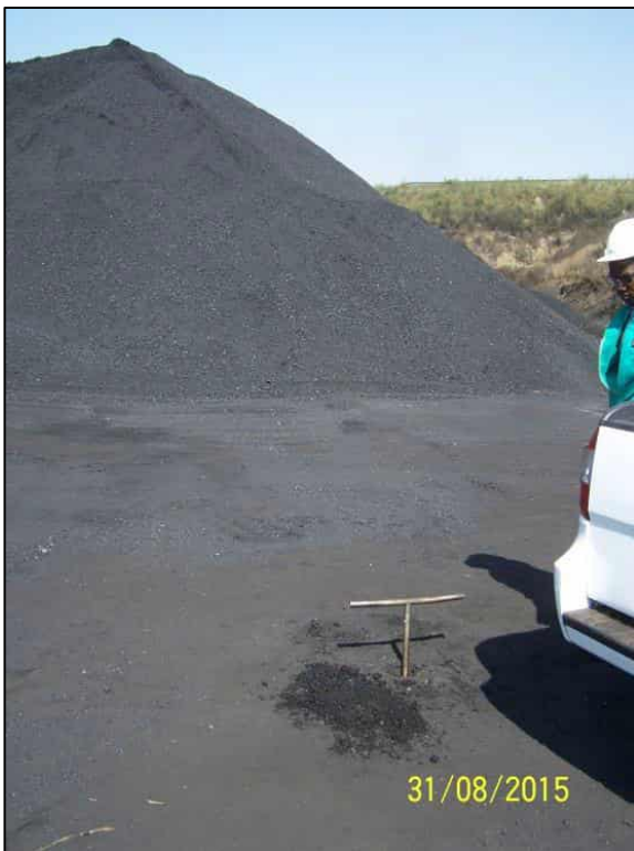
Figure 8: Position of auger sample (Coal stockpile and Ash Dam A in background)
