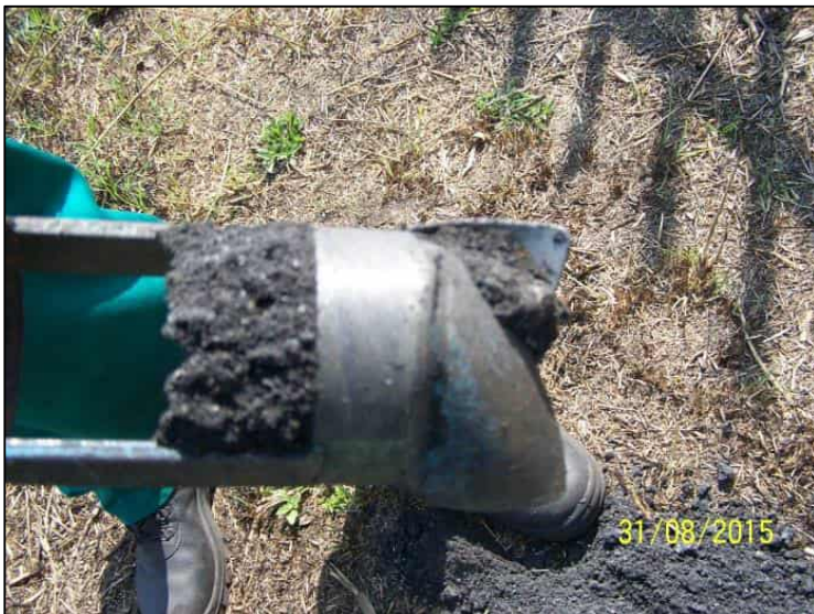
Figure 34: Ash and soil mixture at Pumphouse
