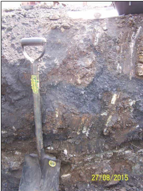
Figure 27: Test pit profile consisting of coal mixed with soil
