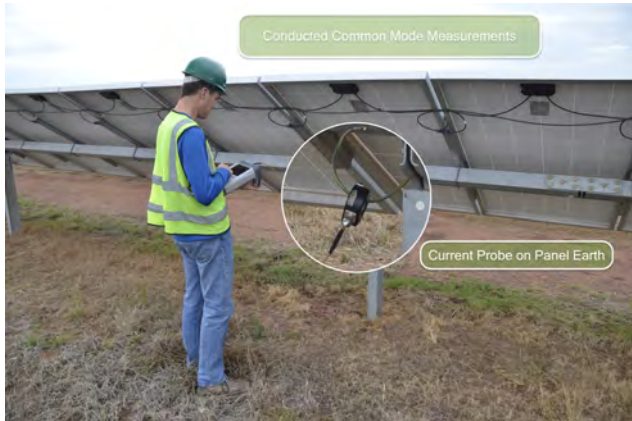
Figure 3: CP measurements on the panel earth strap.
