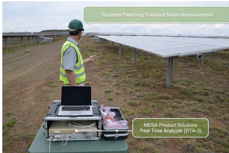
Figure 31: Radiated time domain measurements of Tracking unit.
