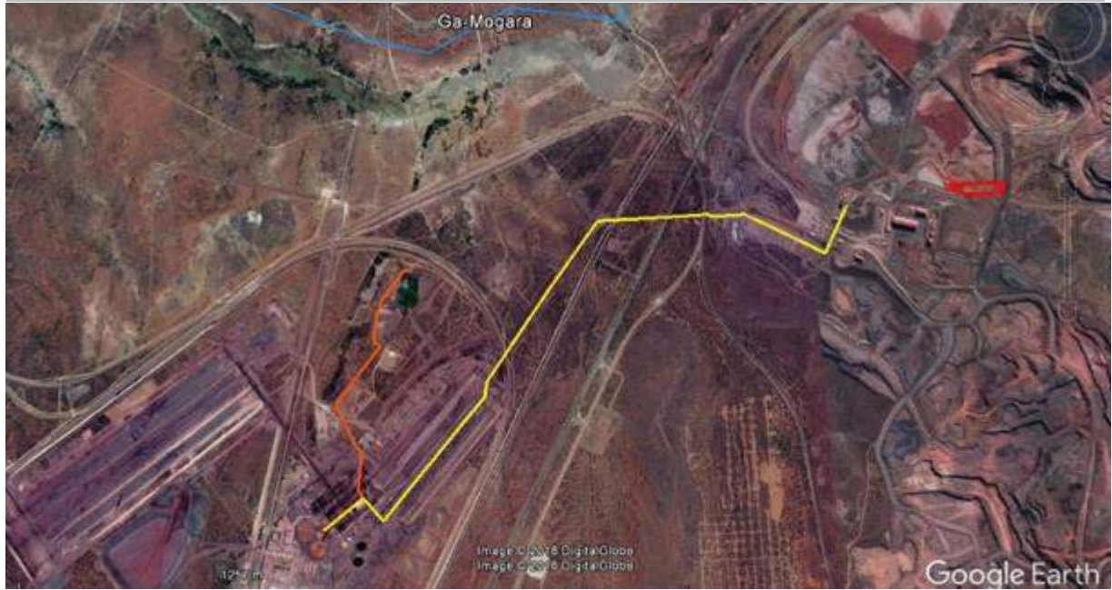
Figure 5: Location of Activities – New Pipelines (yellow – Paste Disposal Facility Return Water Pipeline; orange – Parson Return Water Dam Pipeline)
