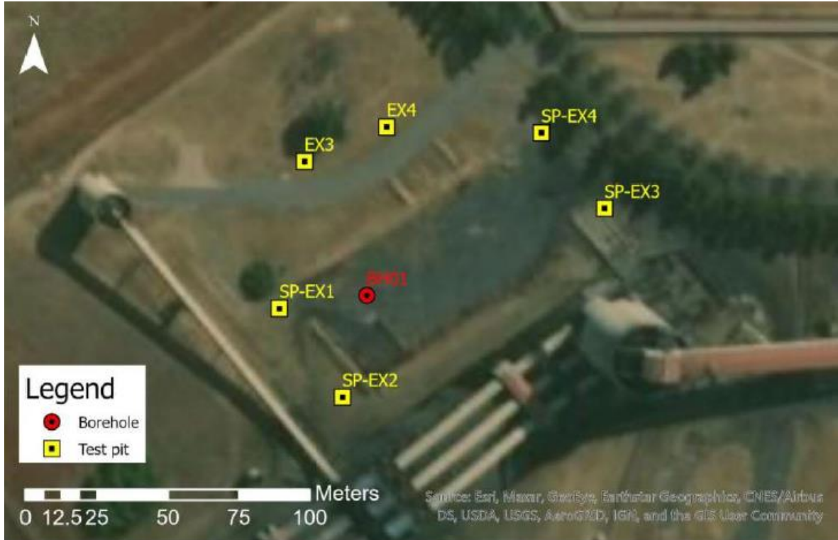
Figure 55: Site plan showing borehole and test pit positions at the ROM Stockpile
