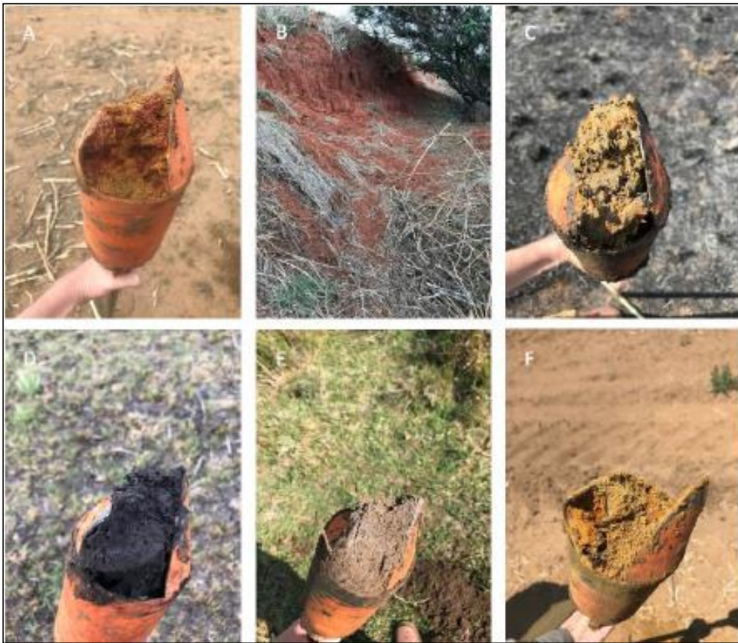
Figure 37: Photographs of selected properties found in the study area – (a) The lithic horizon of Nkonkoni soil form, (b) Profile of the Nkonkoni, (c) Soft plinthic in a profile, (d) Rensburg soils typical of the wetlands in the site, (e) Albic horizon of the Fernwood soil, (f) Lithic horizon of the Clovelly soil
