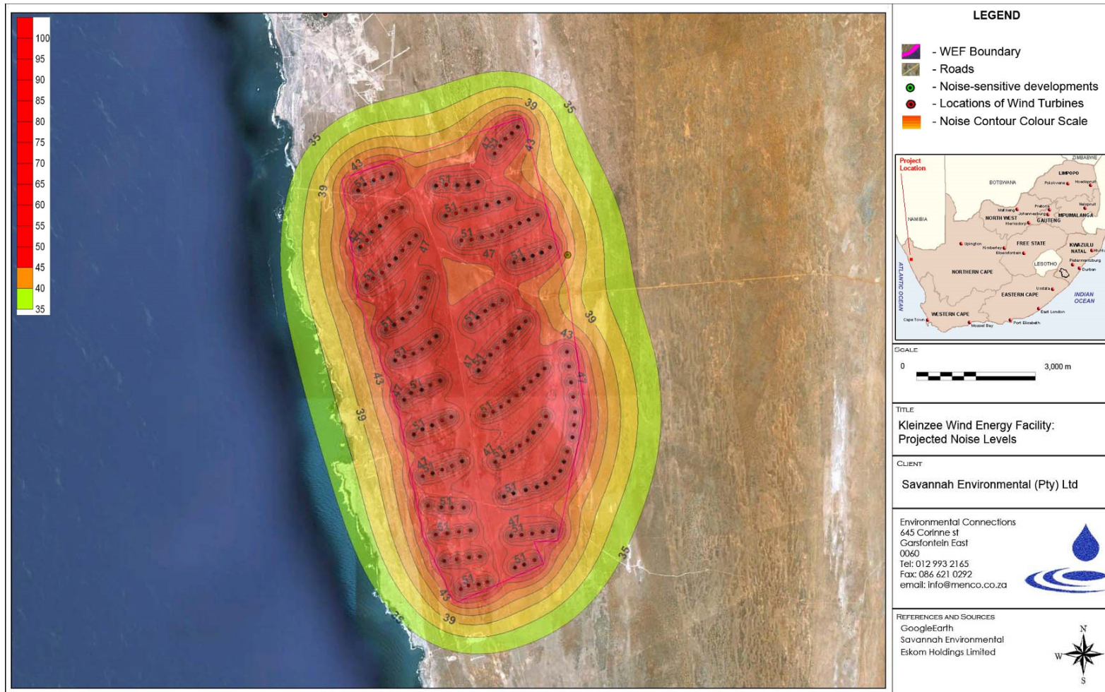
Figure 8.10: Projected Noise Levels (ISO model) from wind turbines; Contours of constant sound levels for a 5 m/s wind
