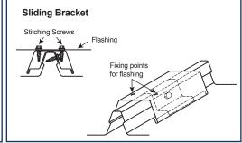
\* When sheet lengths are over 30m flashings must be fixed to sheets using sliding brackets.
