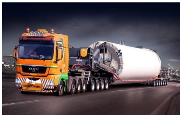
Figure 7-1 Example of Tower Sections Transport (Nooteboom)
