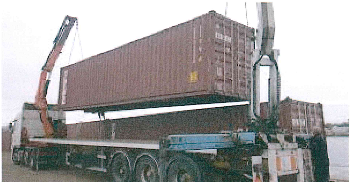
Photo 4: Typical handling and loading of Shipping Containers at Factory and Harbour
