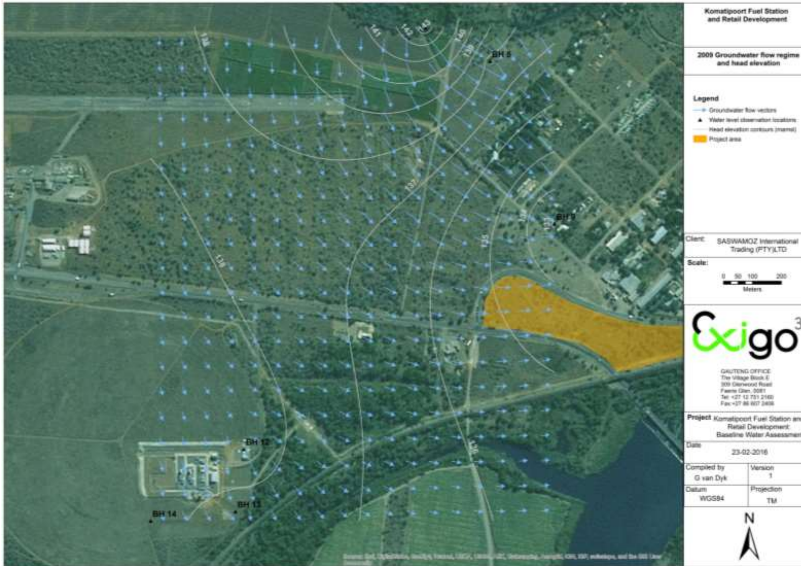
Figure 7 Field survey results and local groundwater regime from water levels taken in 2009
