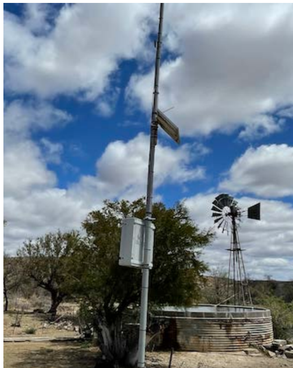
Figure 3: 10 m mast situated close to relatively large trees and an open water source
