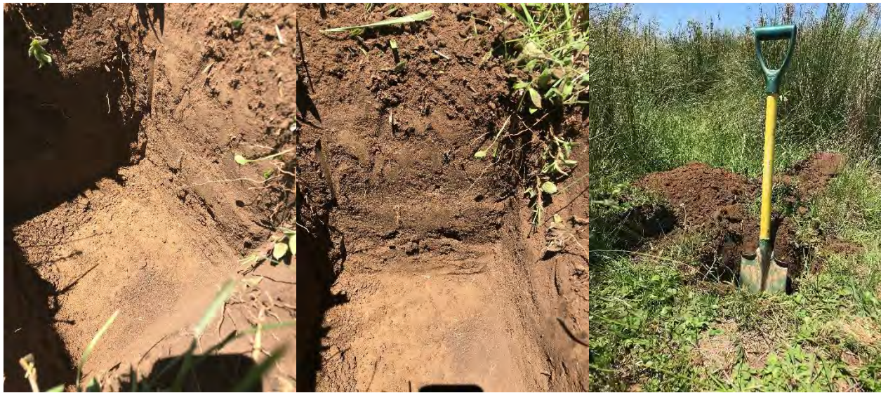
Figure 2: Inspection pits dug to observe in situ soil profiles.
