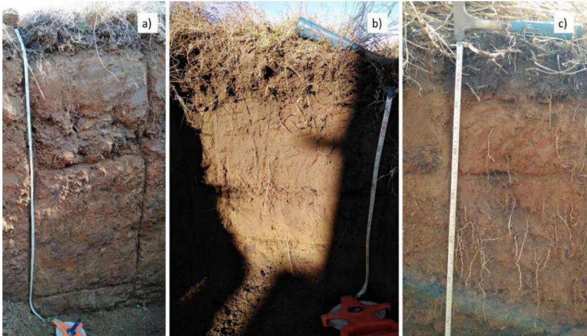
Figure 7-1 Examples of Recharge (deep) soils a) Clovelly, b) Ermelo and c) Lichtenburg.
