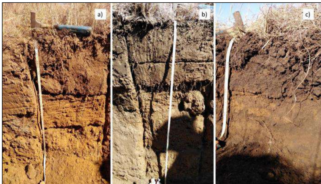
Figure 7-2 Examples of interflow (soil/bedrock) soils a) Avalon, b) Tuluku and c) Inhoek.
