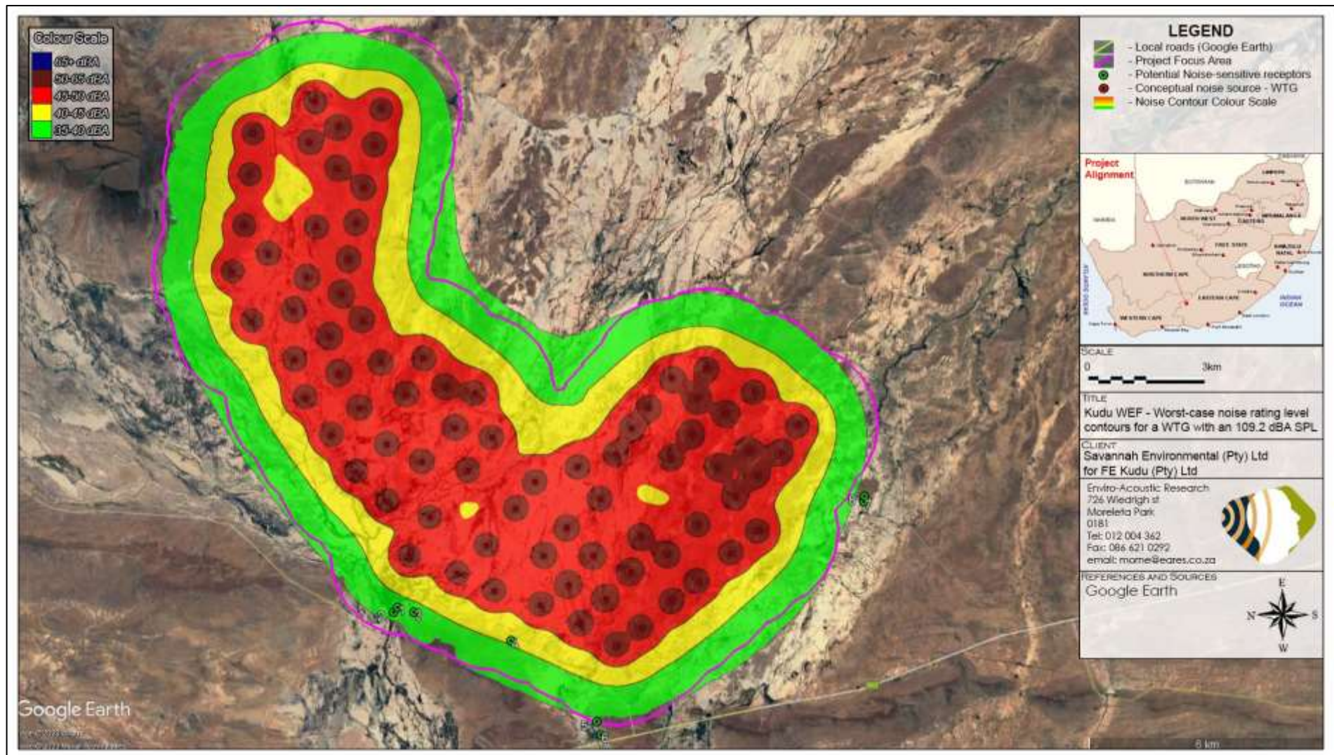
Figure 9-4: Projected future noise rating level contours (worst-case SPL of 109.2 dBA re 1 pW)
