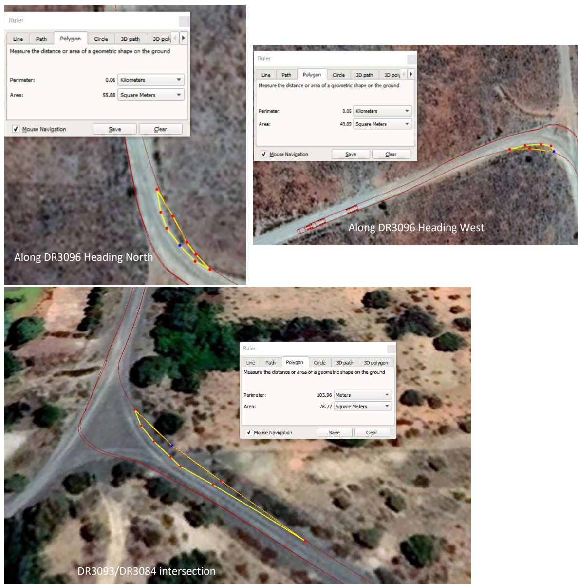
Figure 14-20: Access Route Option 3 Road Widening Requirements
