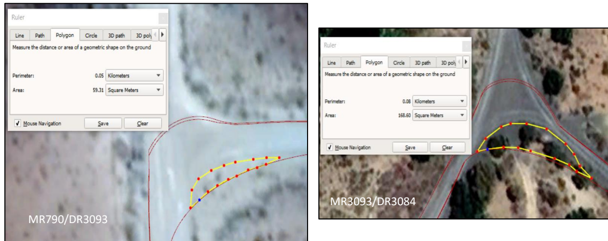
Figure 14-18: Access Route Option 2 Road Widening Requirements
