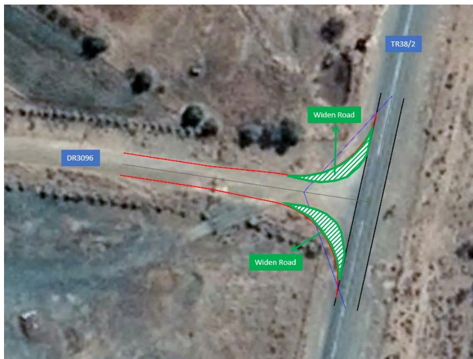
Figure 14-19: Access Route Option 3 Road Widening Requirements
