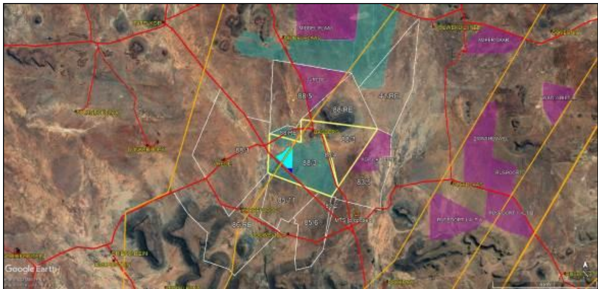
Figure 3.5: Kudu 3 PV site (bold light blue fill), project substation (dark blue fill), and site properties (bold yellow outlines) in relation to adjacent properties (white outlines), proposed Kudu access points (red triangles), other Kudu PV projects (light blue fill), concurrently proposed Crossroads PV Phase 1 sites 21 (pink fill), existing transmission lines (orange), and the existing study area road network (red).
