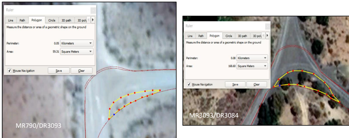
Figure 14-18: Access Route Option 2 Road Widening Requirements
