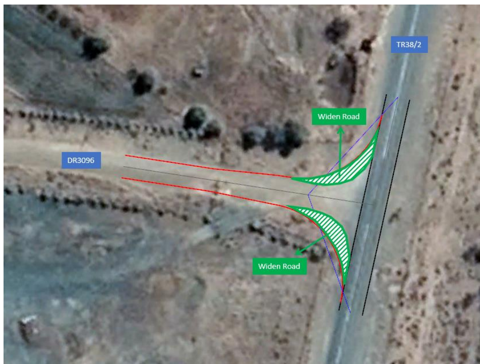
Figure 14-19: Access Route Option 3 Road Widening Requirements
