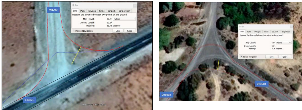
Figure 14-21: Road Widening Width at TR38/01 and MR790 and DR3093 and DR3084 intersections
