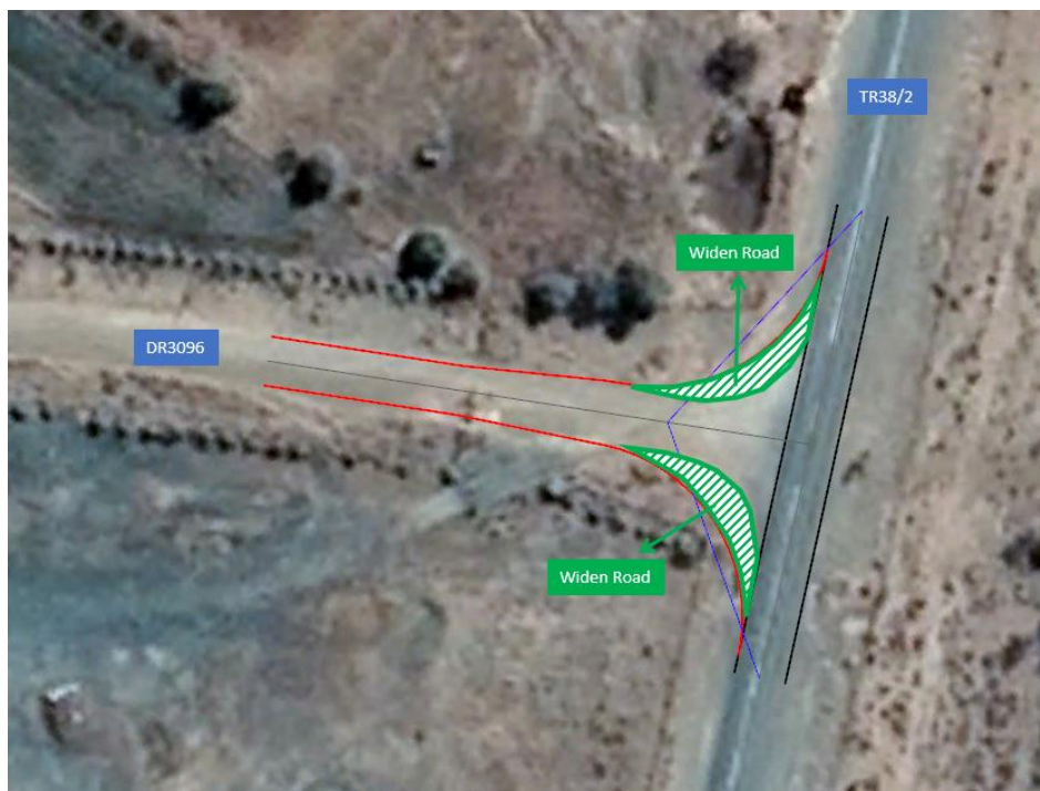
Figure 14-19: Access Route Option 3 Road Widening Requirements
