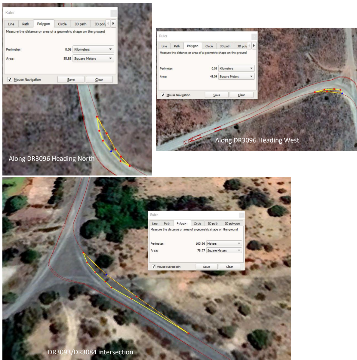
Figure 14-20: Access Route Option 3 Road Widening Requirements
