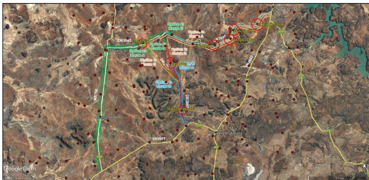
Figure 3.6: Access Route Options (Source: Traffic Impact Assessment for the proposed Kudu Solar Facilities, Sturgeon Consulting, 2023). Red dots indicate dwellings recorded on the relevant 1: 50 000 map rasters; red circles indicate inhabited dwellings <500 m of the road.
