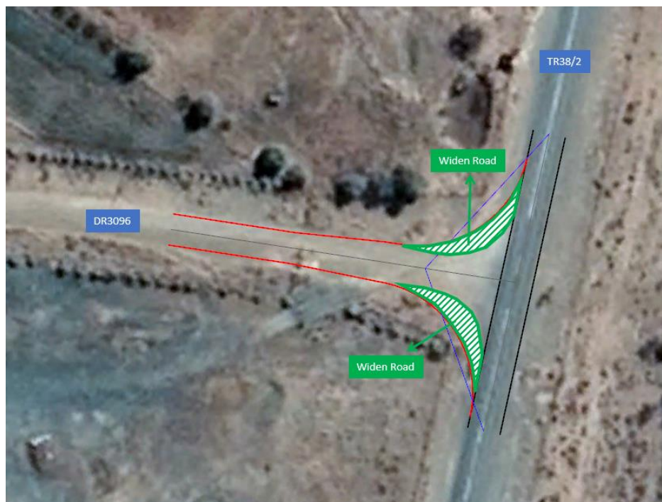
Figure 14-19: Access Route Option 3 Road Widening Requirements
