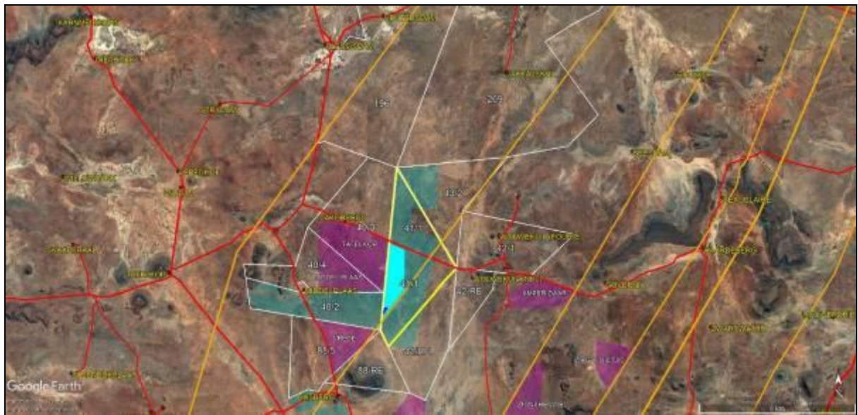
Figure 3.5: Kudu 9 PV site (bold light blue fill), project substation (dark blue fill), and site properties (bold yellow outlines) in relation to adjacent properties (white outlines), proposed Kudu access points (red triangles), other Kudu PV projects (light blue fill), concurrently proposed Crossroads PV Phase 1 sites 21 (pink fill), existing transmission lines (orange), and the study area existing road network (red).
