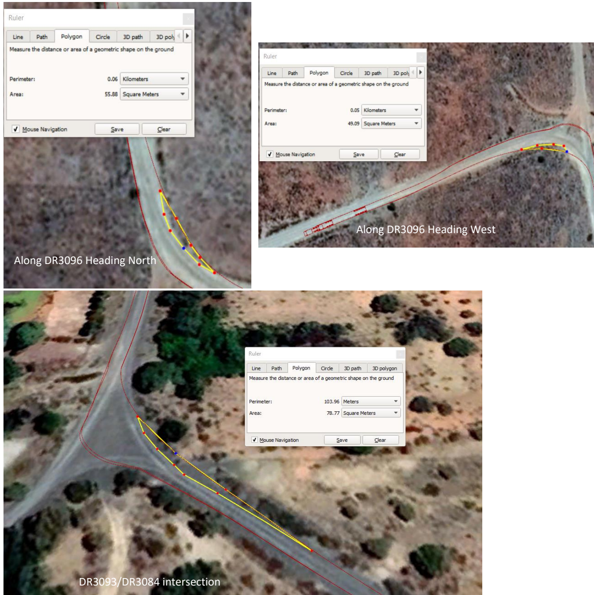
Figure 14-20: Access Route Option 3 Road Widening Requirements
