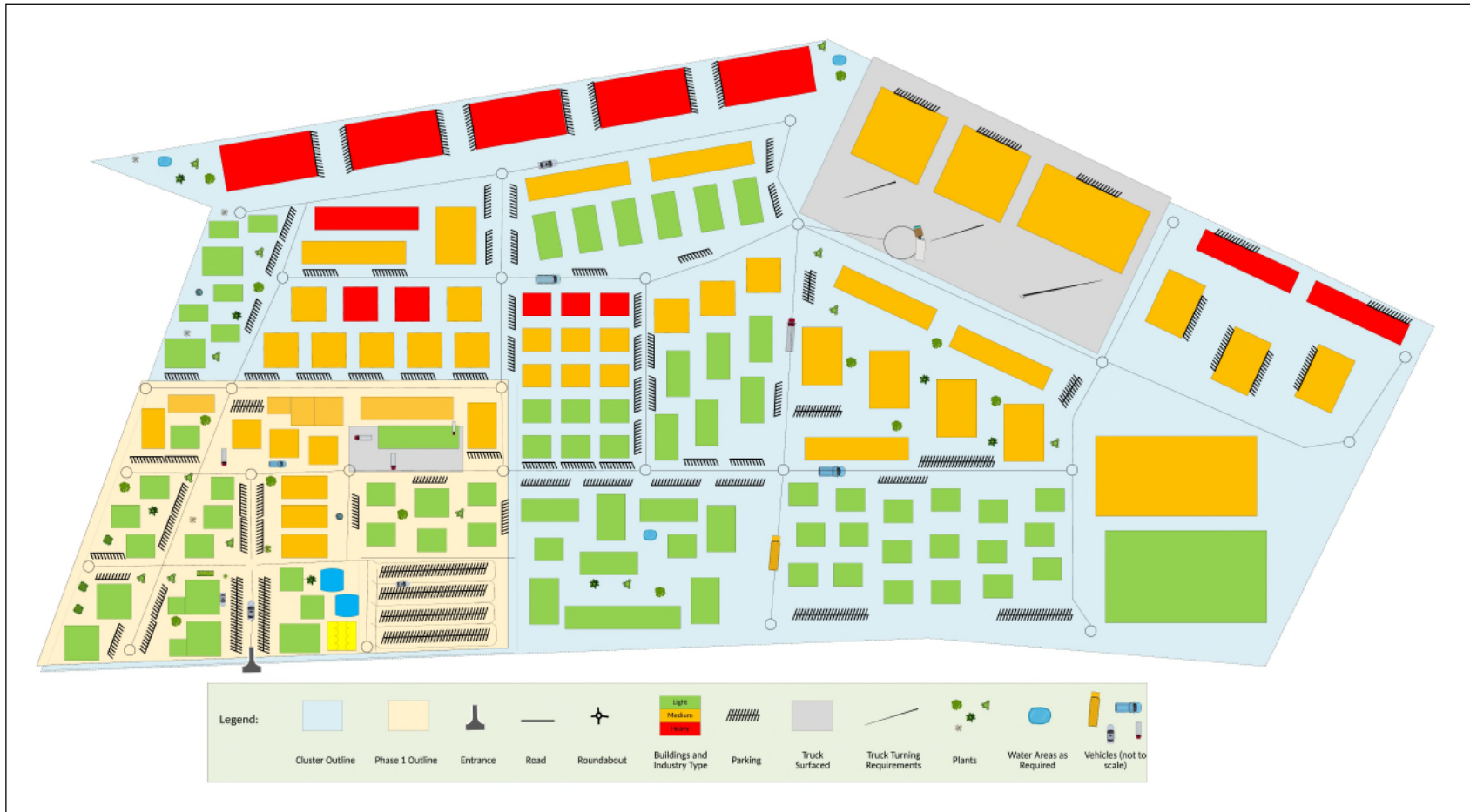
Figure 6.1: Schematic illustration showing a basic layout of the Metals Industrial Cluster located within Portion 6253 of Erf 1, indicating the area earmarked for the Phase 1 development area (refer to Appendix J for an A3 figure)
