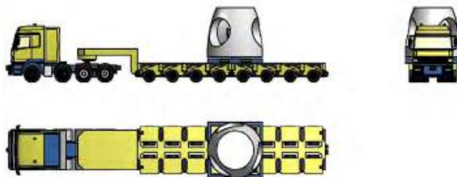
Figure 13: Transporting the Hub and Rotary Units
