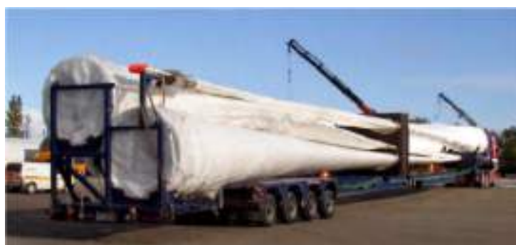
Figure 10: Example: 3 x 45m Blades on extendible trailers
