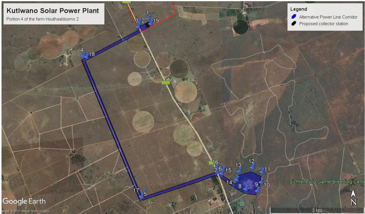
Figure 2.4: Map indicating coordinate points of the proposed Kutlwano Solar Power Plant alternative power line corridor to complete the connection between the collector substation and the existing Watershed MTS enabling evacuation of the power into the national grid.
