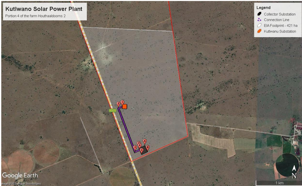
Figure 2.2: Map indicating coordinate points of the proposed Kutlwano Solar Power Plant power line connecting the on-site substation and the collector substation.
