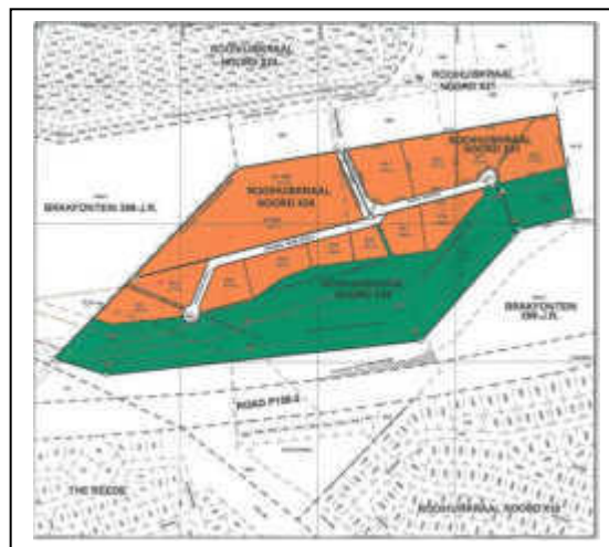
Figure 13c: Alternative layout (Having the proposed development situated on the current Eskom servitude and relocating the Eskom servitude to the south of the site)
