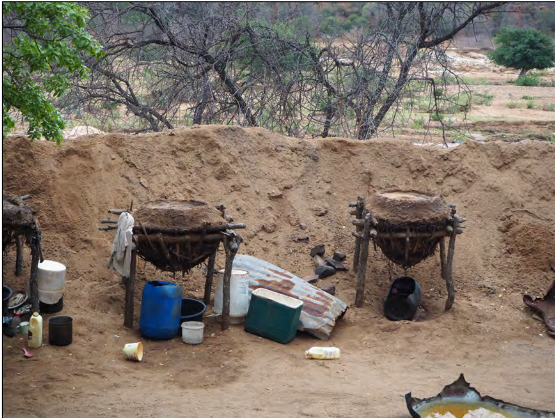
Figure 13. Mopane and Sand Filters
