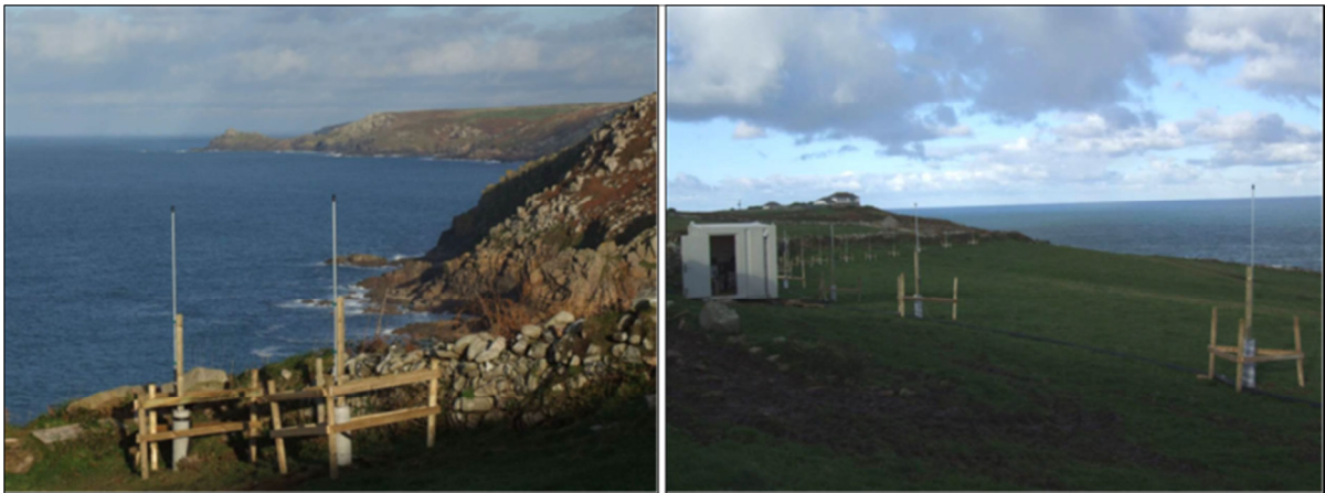
Figure 4.1: Example of the appearance of antennae with “bull-proof” protection and a container at an operational radar station in Cornwall, England (source: Actimar).
