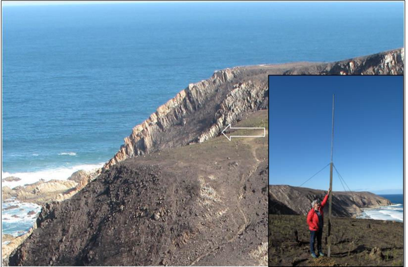
Figure 4.7: The arrow points to a single antenna with guy ropes, erected to demonstrate visibility on one of the South African south coast farms where it is proposed to install the radar. The inset is a close-up image of the same antenna.
