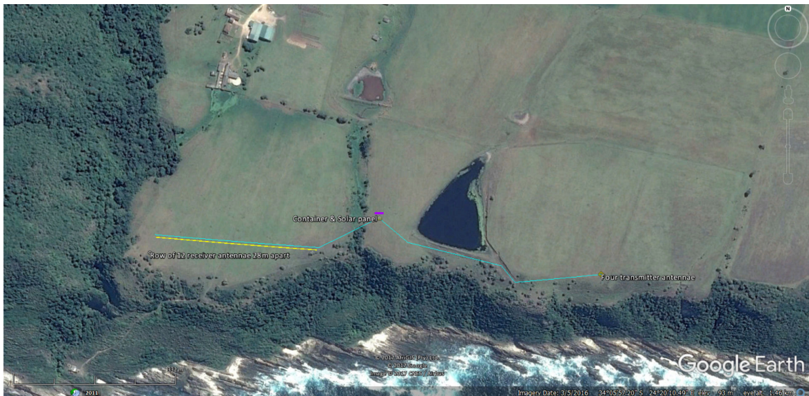
Figure 5.2: Proposed layout of the radar system on Ouwerf farm. The yellow line at bottom left represents a row of 12 receiver antennae placed about 28meters apart, and the small yellow diamond to the right hand side of the image is the 4 transmitter arranged at the corners of a 8.5 x 28.5 rectangle. The blue line shows the route for cables connecting antennae to the container and solar panel at the purple mark towards the centre of the image. The cables can either be buried or laid on the surface as required.
