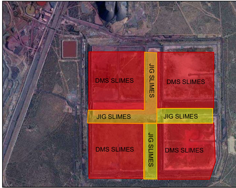
FIGURE 4-5: CURRENT OPERATIONAL LAYOUT OF THE TSF FACILITY
