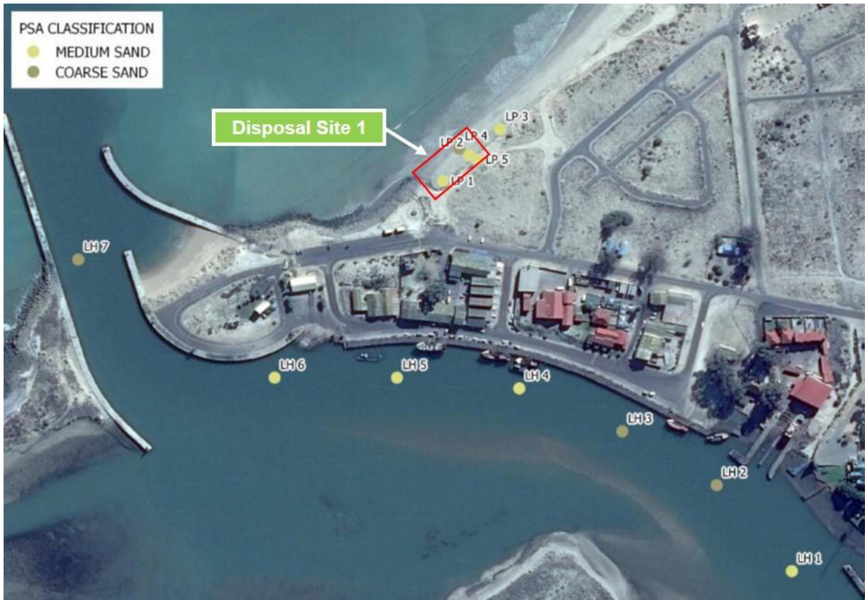
Figure 3-4 Sediment sampling sites in Laaiplek Harbour at the proposed beach nourishment location
