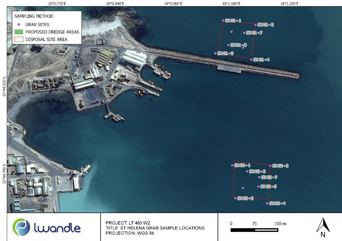
Figure 4-1: Sediment grab sample sites within the two proposed disposal locations for dredge sediments from St Helena Harbour. Sampling was carried out in May 2017.
