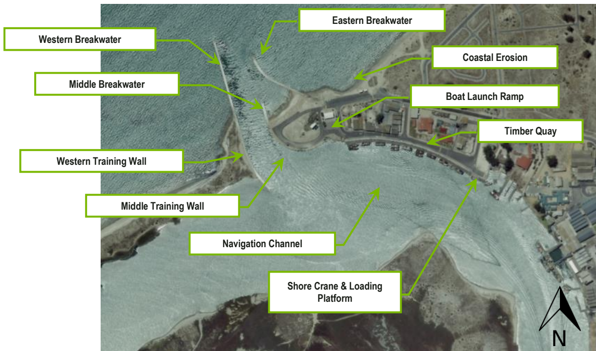
Figure 2-7 Layout and infrastructure of Laaiplek Harbour
