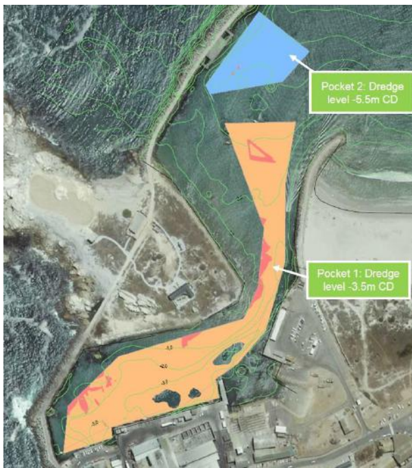
Figure 3-2 Proposed dredging areas in Lamberts Bay harbour showing presence of rock (in red)
