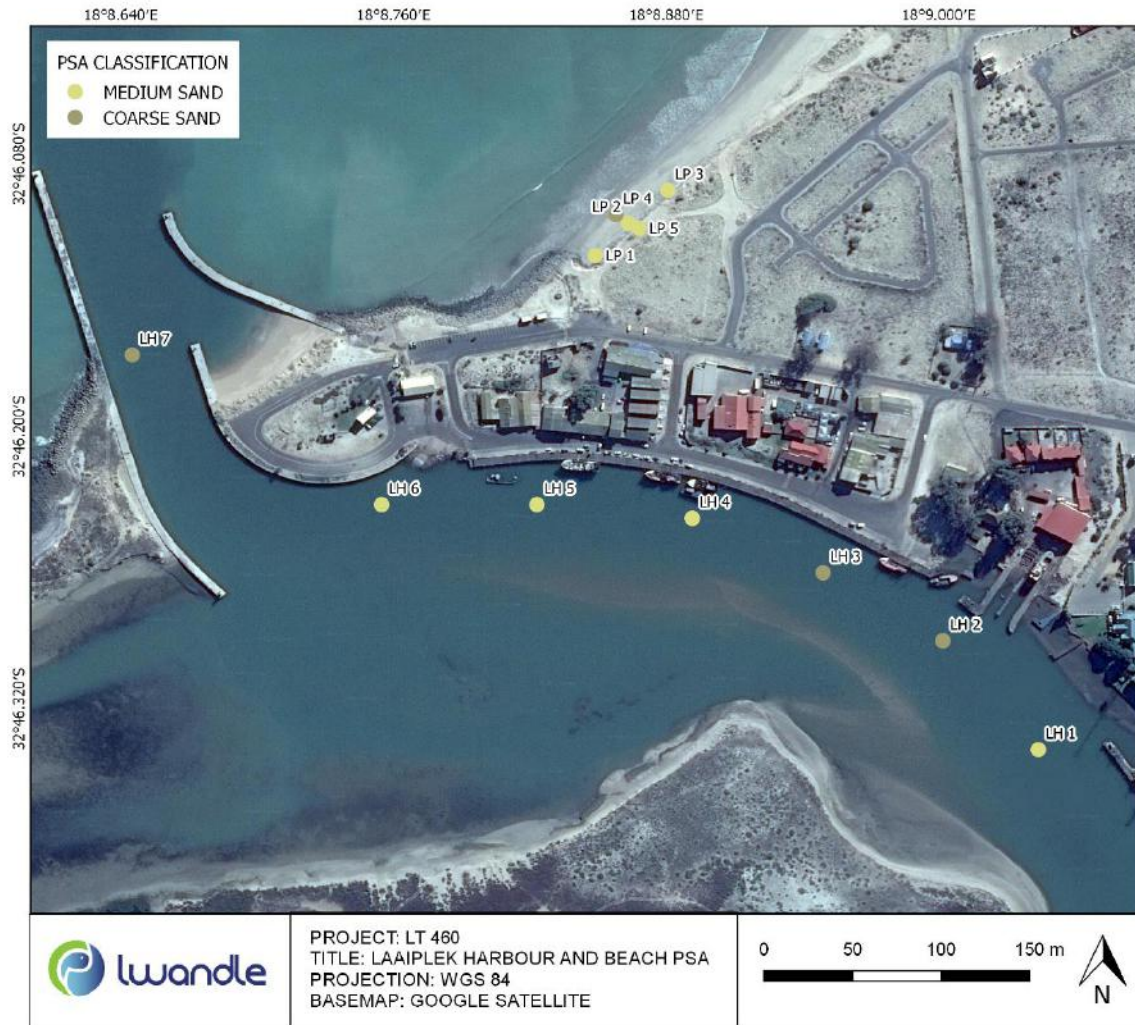
Figure 2-1: Grain size distribution at the dredge sites and the receiving beach north east of the harbour.
