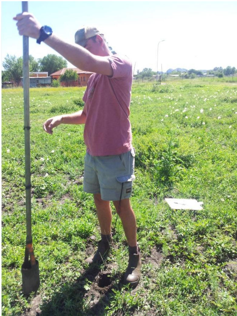
Figure 2. A hand soil augur used for the soil survey.
