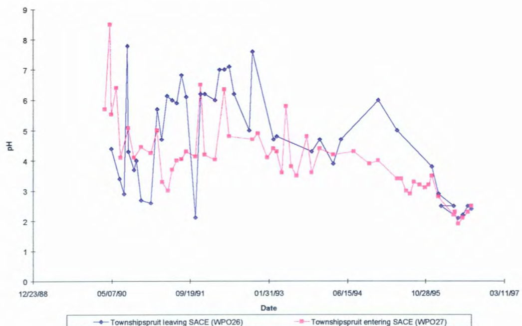
Figure 3.2 (c) Historical pH water quality profile in the Townshipspruit entering and leaving the SACE property
