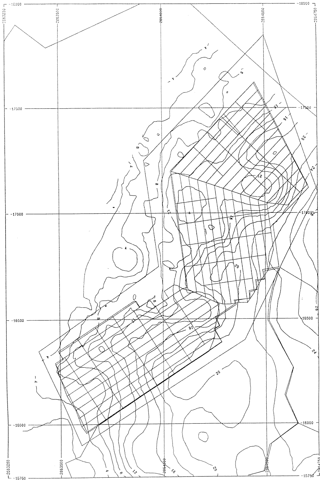
FIGURE 3: OVERBURDEN DEPTH CONTOURS FOR THE SCHOONGEZICHT MINI-PIT PRESENTED IN INTERVALS OF 2m.
