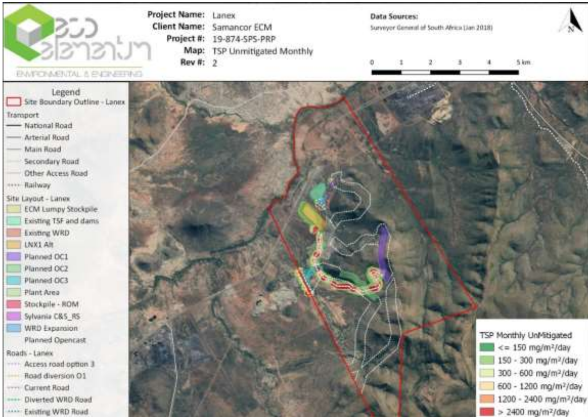
Figure 8-66: Predicted highest monthly deposition for TSP for the proposed Lannex Operations when unmitigated
