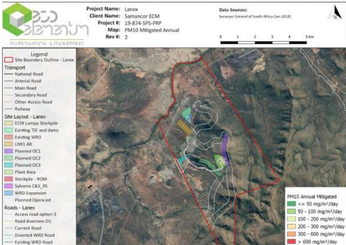
Figure 8-61: Predicted average annual concentrations for PM 10 for the proposed Lannex Project operations when mitigated
