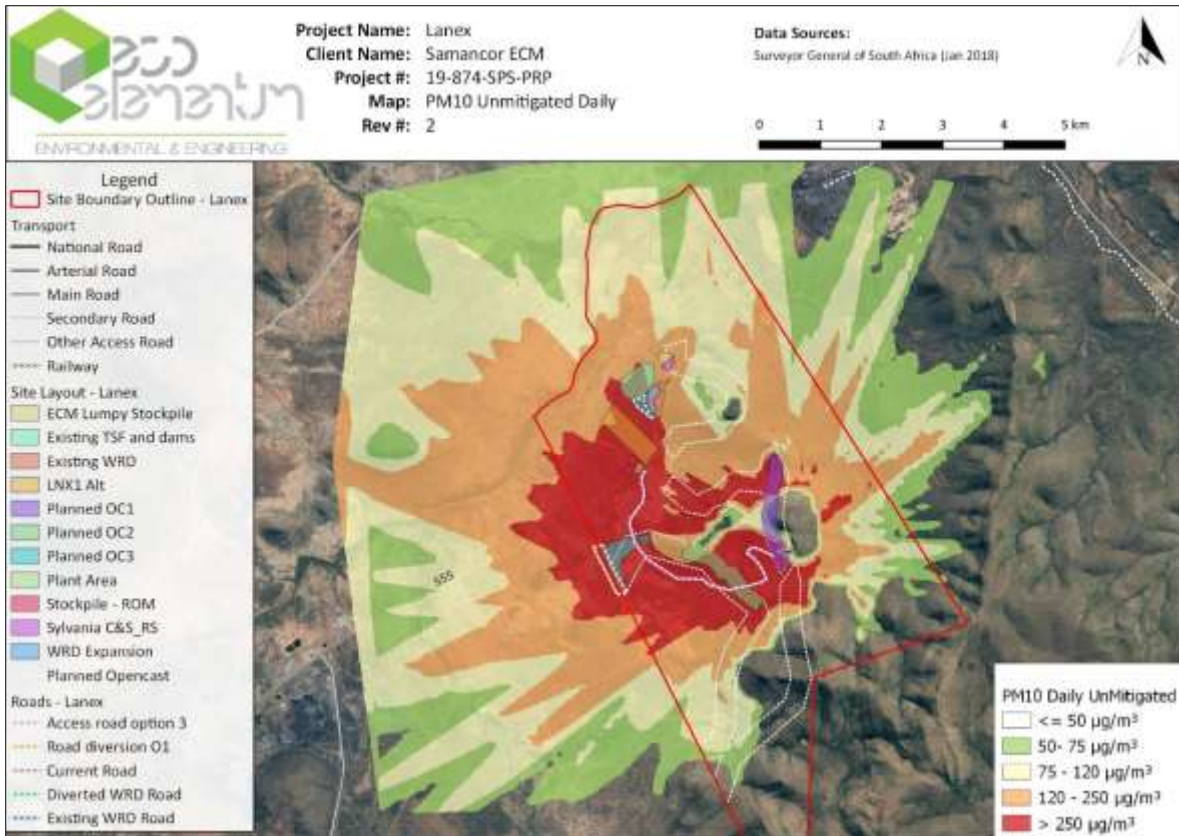
Figure 8-62: Predicted 2 nd Highest daily concentrations for PM 10 for the proposed Lannex project when unmitigated
