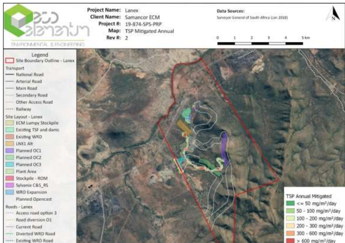
Figure 8-65: Predicted average annual deposition for TSP for the proposed Lannex operations when mitigated
