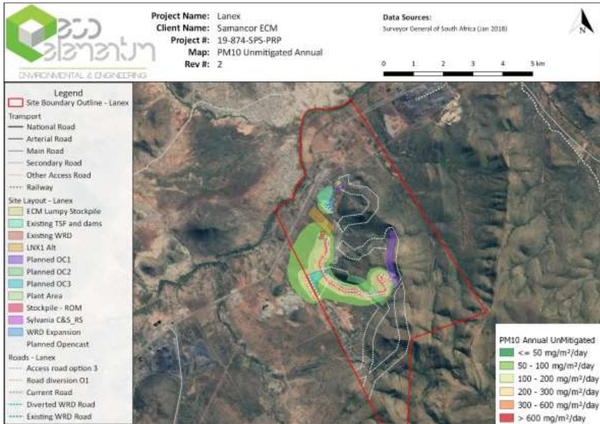
Figure 8-60: Predicted average annual concentrations for PM 10 for the proposed Lannex project when unmitigated
