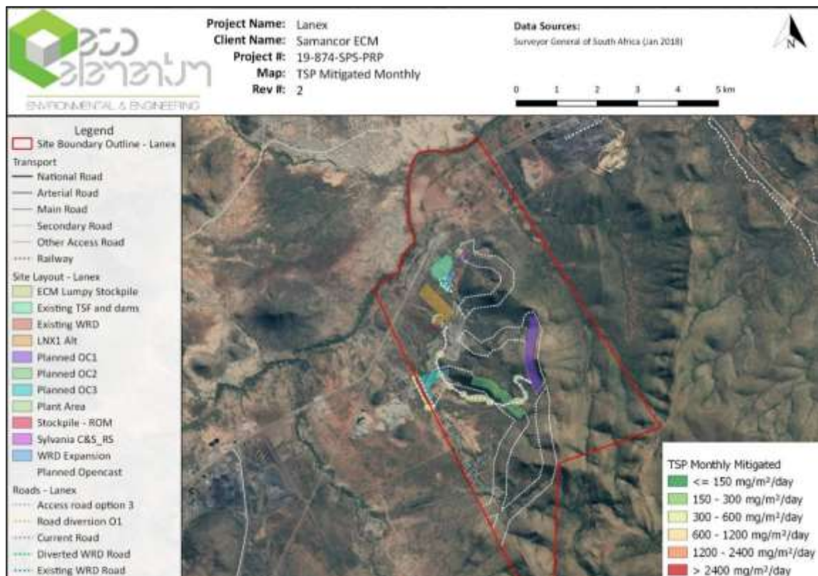
Figure 8-67: Predicted highest monthly deposition for TSP for the proposed Lannex project operations when mitigated
