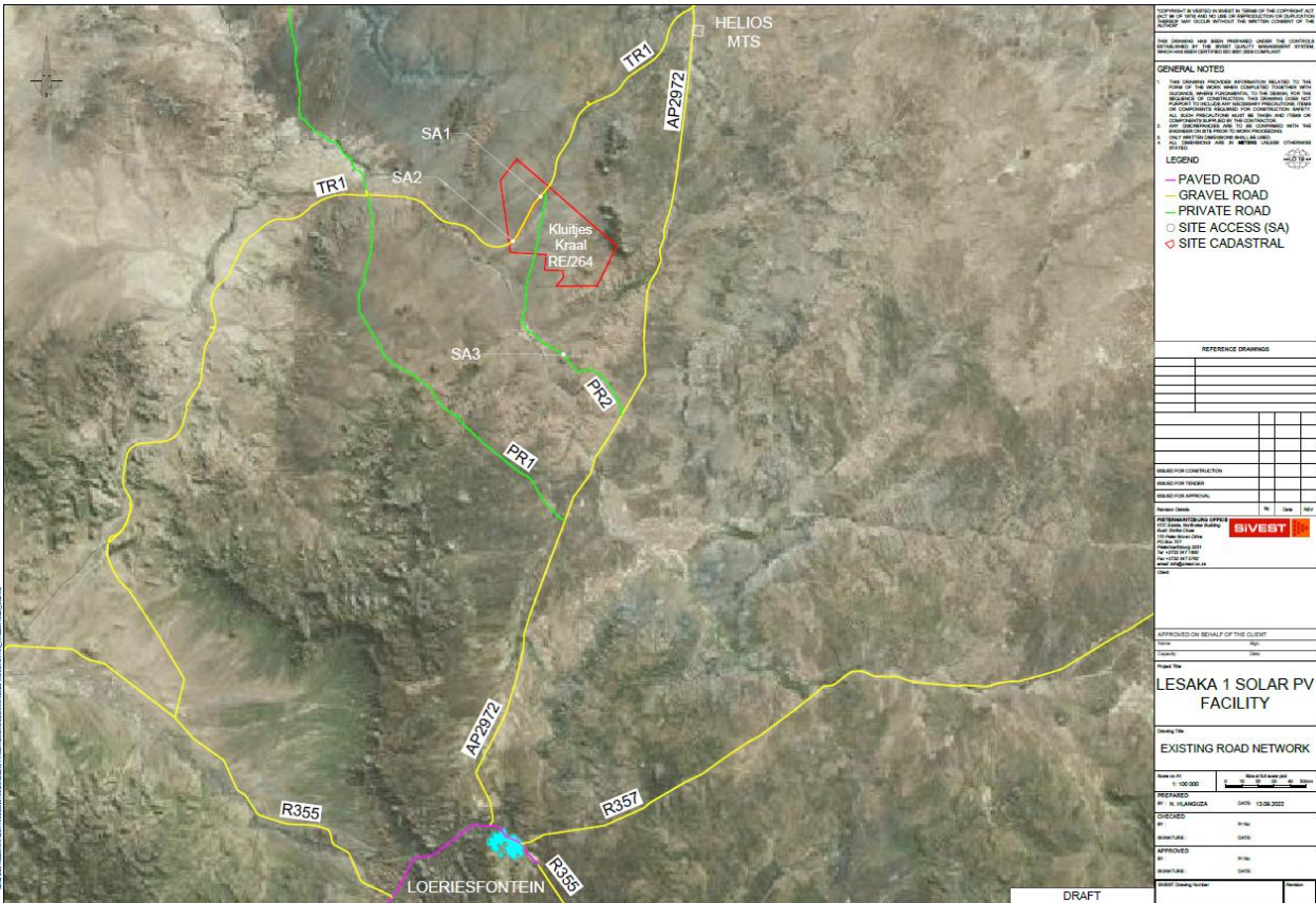
Figure 5-5 External Road Network
