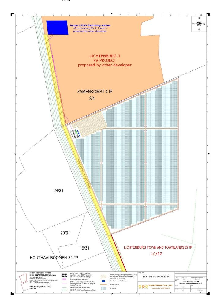
Figure 2. Proposed Draft Layout Plan of the Lichtenburg Solar Park – Alternative 2
