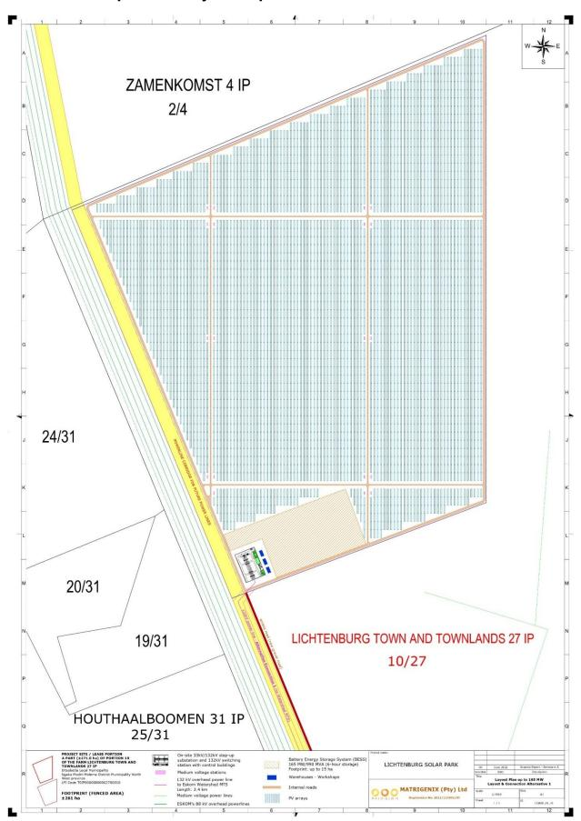
Figure 1. Proposed Draft Layout Plan of the Lichtenburg Solar Park – Alternative 1 (Preferred)
