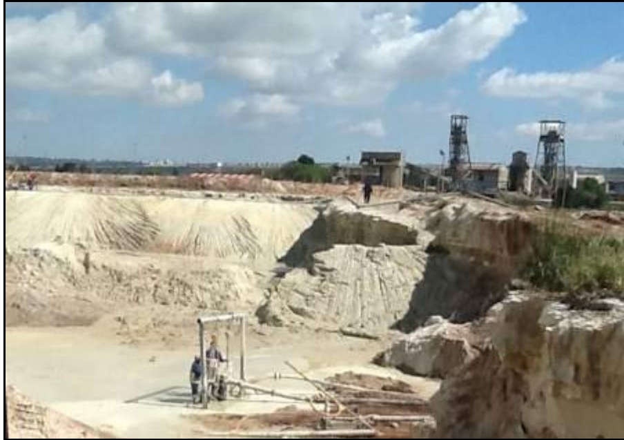
Figure 22: Typical Hydraulic mining technique being used to mine tailings
