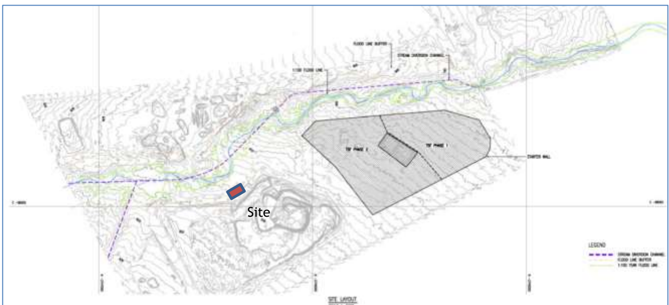
Figure 3-7: 1:100 year flood line for the Steelpoort River (extracted from Knight Piésold Consulting, 2019)
