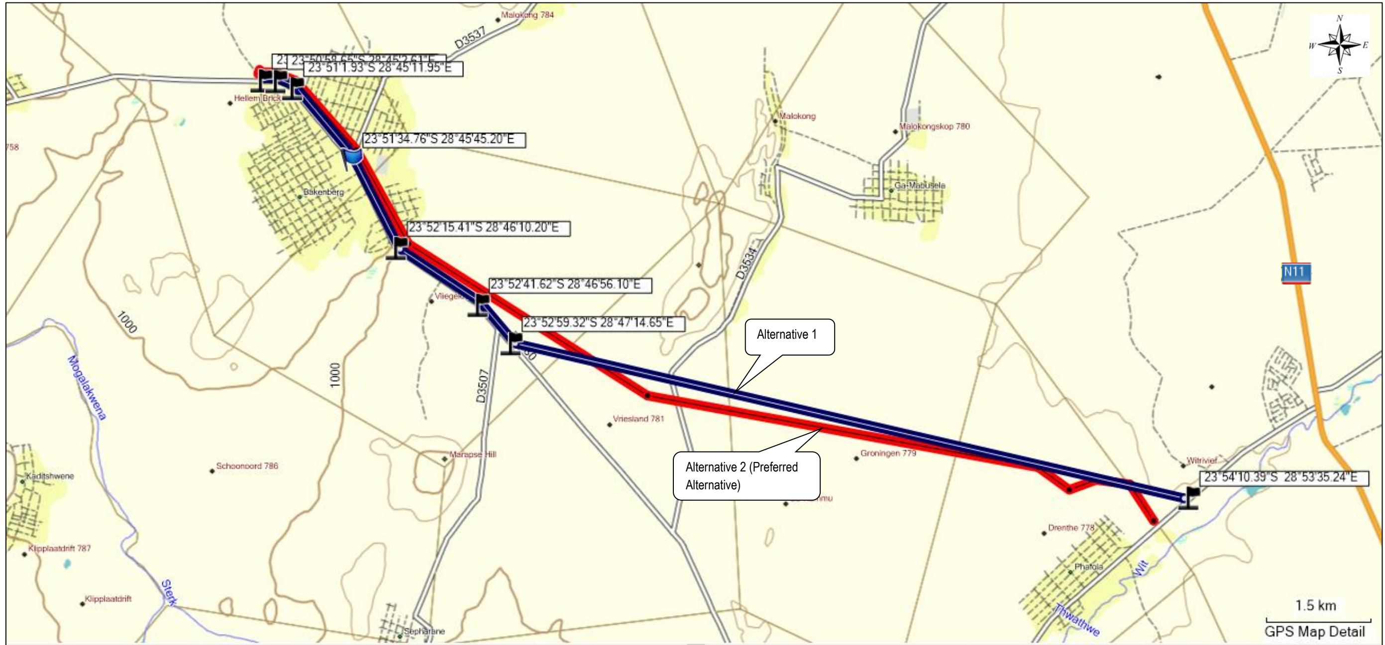
Locality Map: Proposed 16,6km, 600mm diameter water pipeline, with a throughput of 271.10l/s linking existing pipelines near Witrivier/Phafola to Bakenberg.
