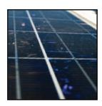
Amorphous Silicon - Amorphous silicon is the noncrystalline form of silicon and was the first thin film material to yield a commercial product, first used in consumer items such as calculators. It can be deposited in thin layers onto a variety of surfaces and offers lower costs than traditional crystalline silicon, though it is less efficient at converting sunlight into electricity.
