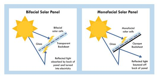
Figure 5.3: Bifacial vs Monoficial Solar Panel absorption.
