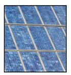
Poly-crystalline Silicon – poly-crystalline panels use solar cells that are cut from multifaceted silicon crystals. They are less uniform in appearance than mono-crystalline cells, resembling pieces of shattered glass. These are the most common solar panels on the market, being less expensive than mono-crystalline silicon. They are also less efficient, though the performance gap has begun to close in recent years (First Solar, 2011).
