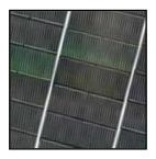
Copper, Indium, Gallium, Selenide (CIGS) - CIGS is a compound semiconductor that can be deposited onto many different materials. CIGS has only recently become available for small commercial applications, and is considered a developing PV technology (First Solar, 2011).
