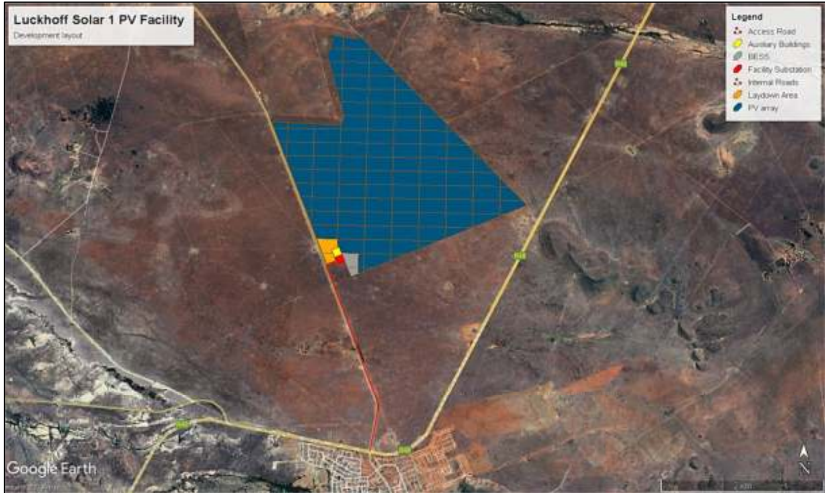
Figure 5.3: Final layout plan for the Luckhoff Solar 1 PV facility and associated infrastructure
