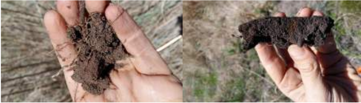
Figure 13: Iron precipitation along roots indicating a fluctuating water table
