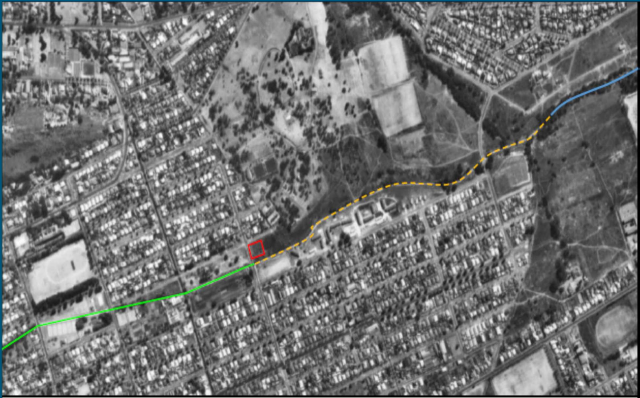
Figure 24: Extensive Development, Canalised Portion of the Jukskei River (Orange) Natural Watercourse (blue line) and Underground Portion of the Canal (Green)
