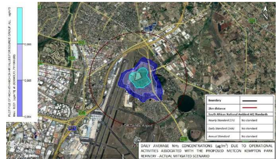
Figure 5-39: Predicted NH 3 daily average incremental concentrations for the proposed MetCon Jewellery Precinct facility – Actual mitigated scenario.
