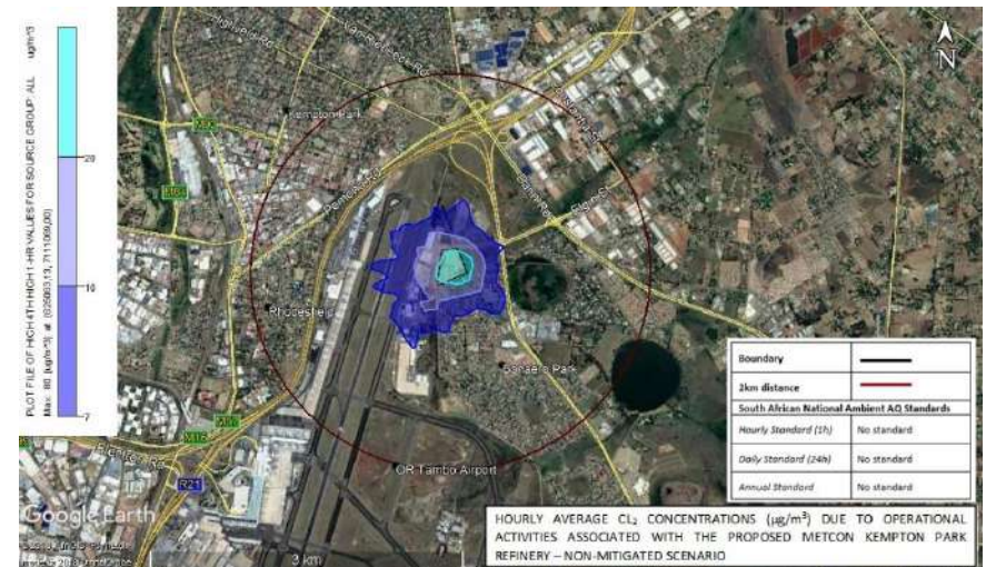
Figure 5-20: Predicted CL 2 hourly average incremental concentrations for the proposed MetCon Jewellery Precinct facility – Unmitigated scenario.
