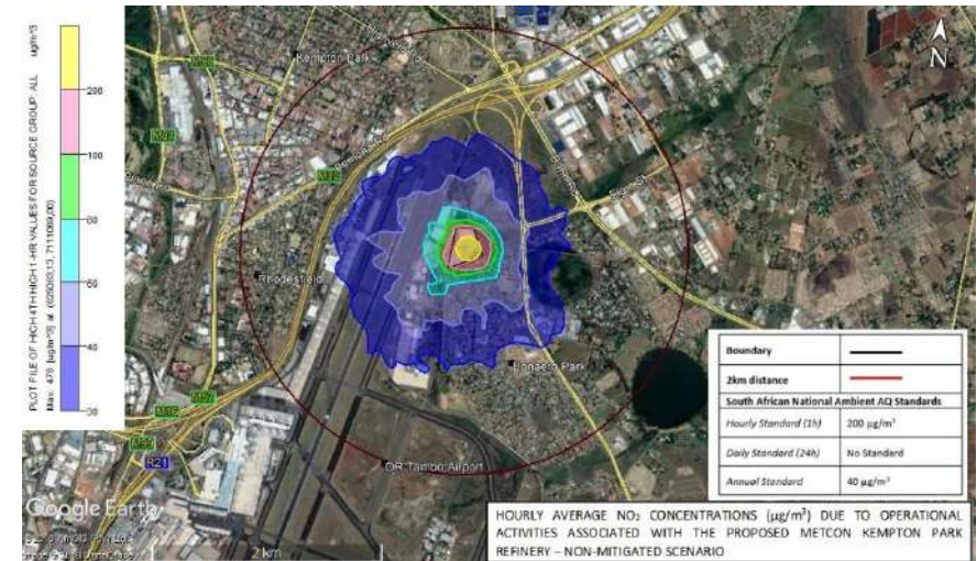
Figure 5-16: Predicted NO 2 hourly average incremental concentrations for the proposed MetCon Jewellery Precinct facility – Unmitigated scenario.
