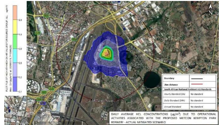
Figure 5-27: Predicted HCL daily average incremental concentrations for the proposed MetCon Jewellery Precinct facility – Actual mitigated scenario.
