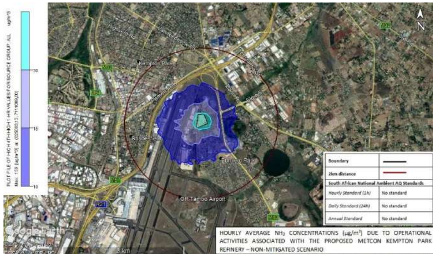
Figure 5-38: Predicted NH 3 hourly average incremental concentrations for the proposed MetCon Jewellery Precinct facility – Unmitigated scenario.
