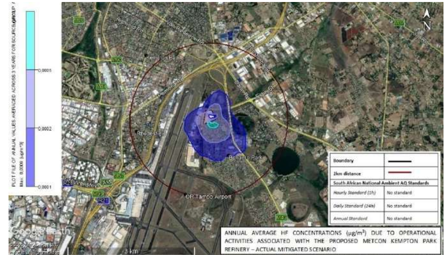
Figure 5-35: Predicted HF annual average incremental concentrations for the proposed MetCon Jewellery Precinct facility – Actual mitigated scenario.
