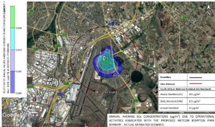
Figure 5-13: Predicted SO 2 annual average incremental concentrations for the proposed MetCon Jewellery Precinct facility – Actual mitigated scenario.
