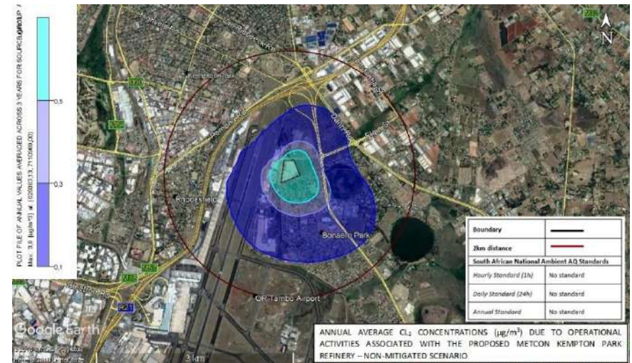
Figure 5-24: Predicted CL 2 annual average incremental concentrations for the proposed MetCon Jewellery Precinct facility – Unmitigated scenario.
