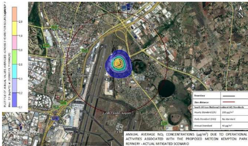
Figure 5-17: Predicted NO 2 annual average incremental concentrations for the proposed MetCon Jewellery Precinct facility – Actual mitigated scenario.
