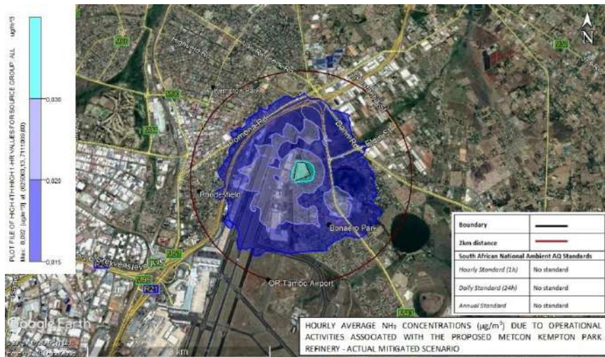
Figure 5-37: Predicted NH 3 hourly average incremental concentrations for the proposed MetCon Jewellery Precinct facility – Actual mitigated scenario.
