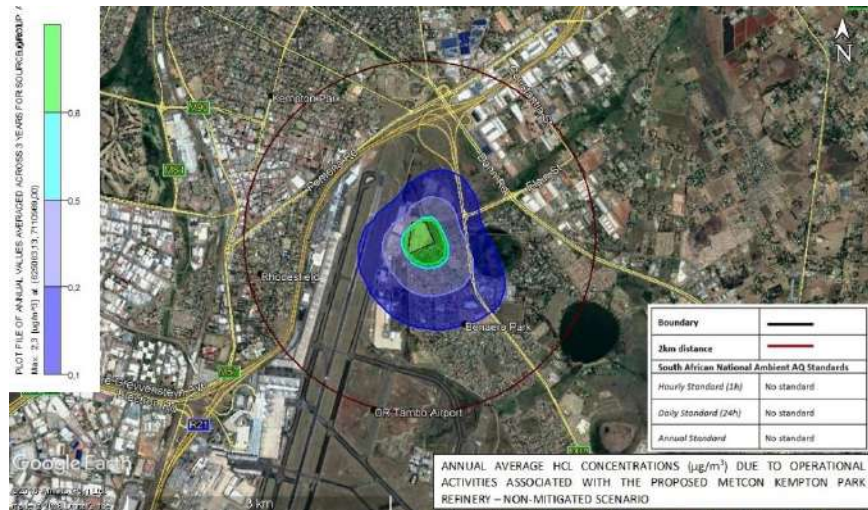
Figure 5-30: Predicted HCL annual average incremental concentrations for the proposed MetCon Jewellery Precinct facility – Unmitigated scenario.
