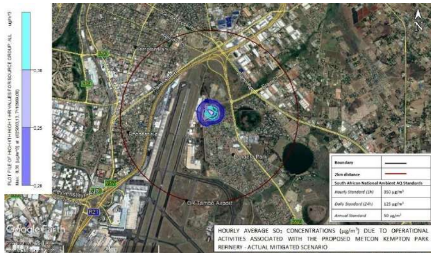
Figure 5-9: Predicted SO 2 hourly average incremental concentrations for the proposed MetCon Jewellery Precinct facility – Actual mitigated scenario.
