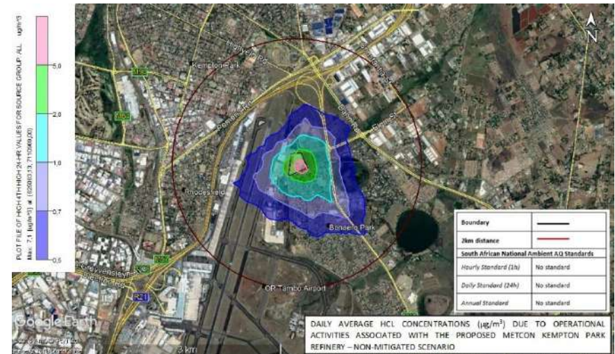
Figure 5-28: Predicted HCL daily average incremental concentrations for the proposed MetCon Jewellery Precinct facility – Unmitigated scenario.
