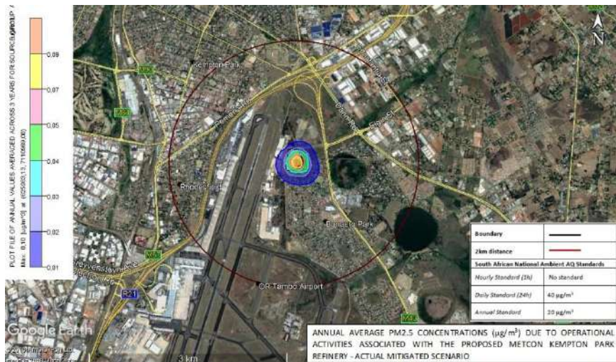
Figure 5-6: Predicted PM 2.5 annual average incremental concentrations for the proposed MetCon Jewellery Precinct facility – Actual mitigated scenario.
