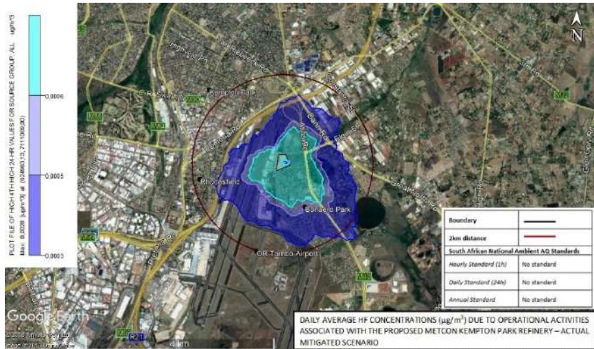
Figure 5-33: Predicted HF daily average incremental concentrations for the proposed MetCon Jewellery Precinct facility – Actual mitigated scenario.
