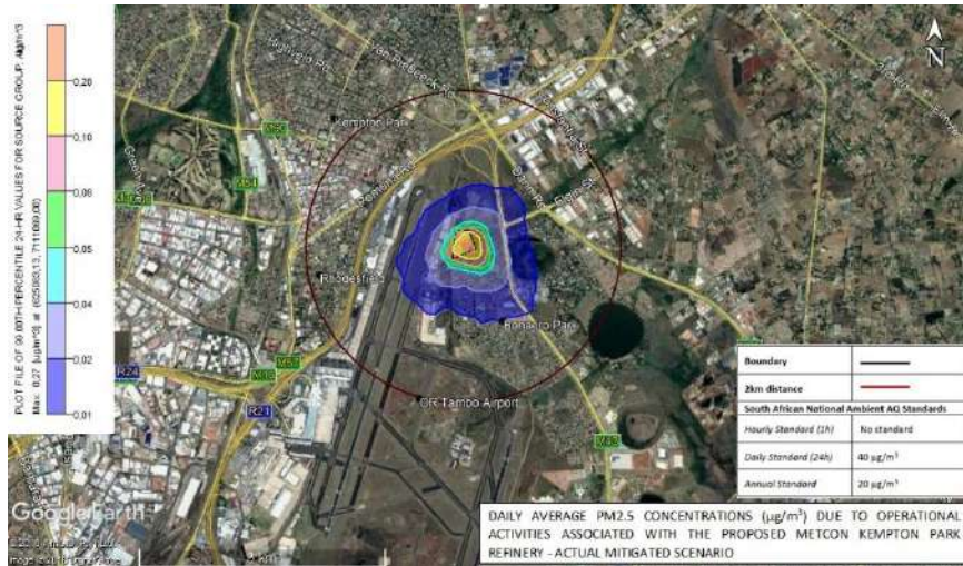
Figure 5-5: Predicted PM 2.5 daily average incremental concentrations for the proposed MetCon Jewellery Precinct facility – Actual mitigated scenario.
