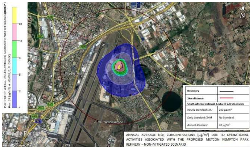
Figure 5-18: Predicted NO 2 annual average incremental concentrations for the proposed MetCon Jewellery Precinct facility – Unmitigated scenario.
