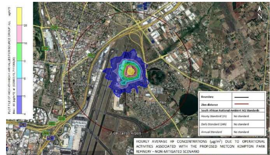
Figure 5-32: Predicted HF hourly average incremental concentrations for the proposed MetCon Jewellery Precinct facility – Unmitigated scenario.
