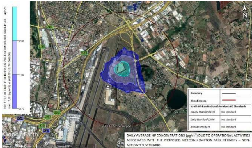
Figure 5-34: Predicted HF daily average incremental concentrations for the proposed MetCon Jewellery Precinct facility – Unmitigated scenario.
