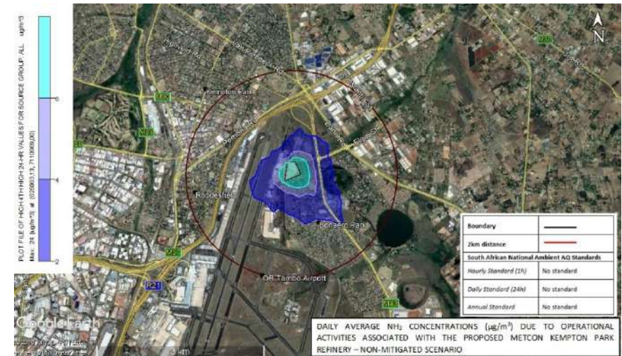
Figure 5-40: Predicted NH 3 daily average incremental concentrations for the proposed MetCon Jewellery Precinct facility – Unmitigated scenario.
