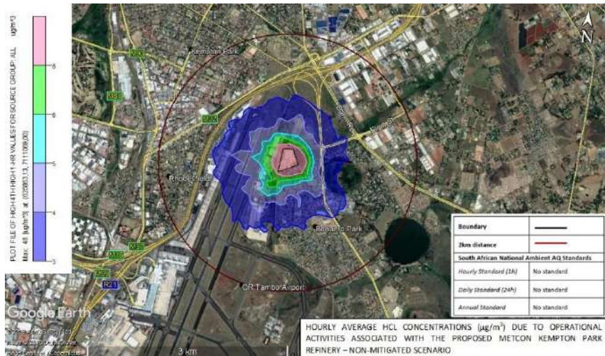
Figure 5-26: Predicted HCL hourly average incremental concentrations for the proposed MetCon Jewellery Precinct facility – Unmitigated scenario.
