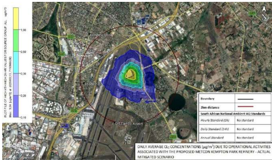
Figure 5-21: Predicted CL 2 daily average incremental concentrations for the proposed MetCon Jewellery Precinct facility – Actual mitigated scenario.
