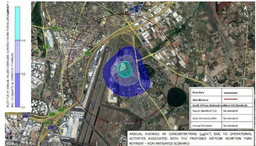
Figure 5-36: Predicted HF annual average incremental concentrations for the proposed MetCon Jewellery Precinct facility – Unmitigated scenario.
