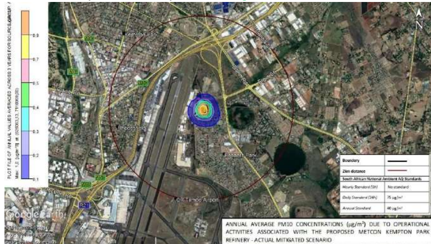
Figure 5-2: Predicted PM 10 annual average incremental concentrations for the proposed MetCon Jewellery Precinct facility – Actual mitigated scenario.
