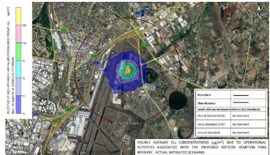
Figure 5-19: Predicted CL 2 hourly average incremental concentrations for the proposed MetCon Jewellery Precinct facility – Actual mitigated scenario.
