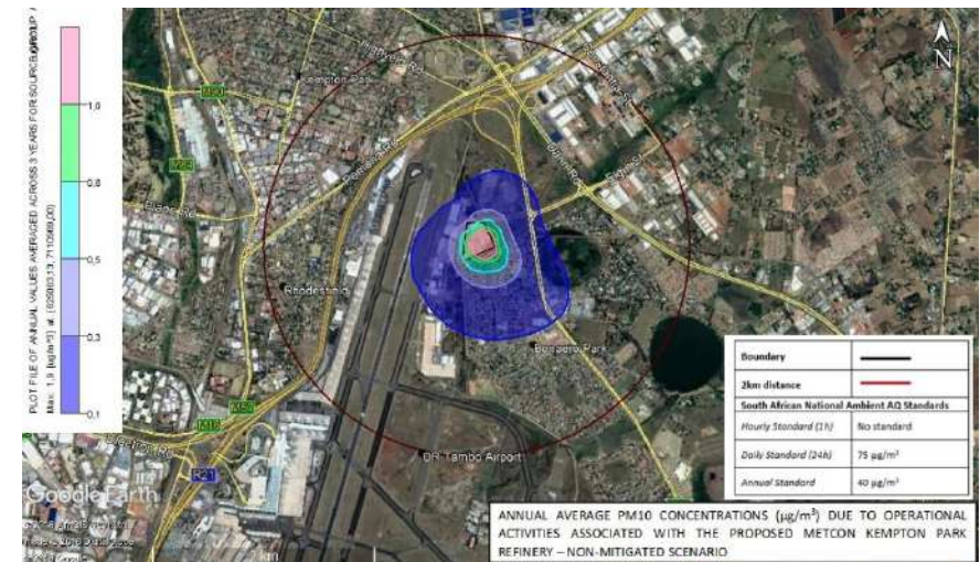
Figure 5-4: Predicted PM 10 annual average incremental concentrations for the proposed MetCon Jewellery Precinct facility – Unmitigated scenario.
