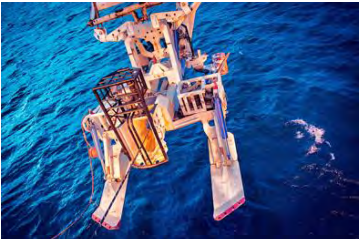
Figure 2-19 Elettra – Taurus 2 SMD Plough System
