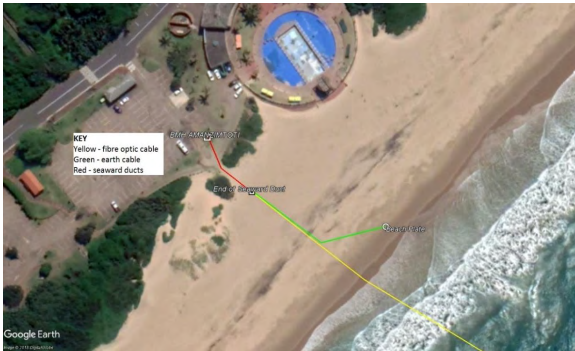
Figure 2-7 Proposed Beach Earth Plate Location
