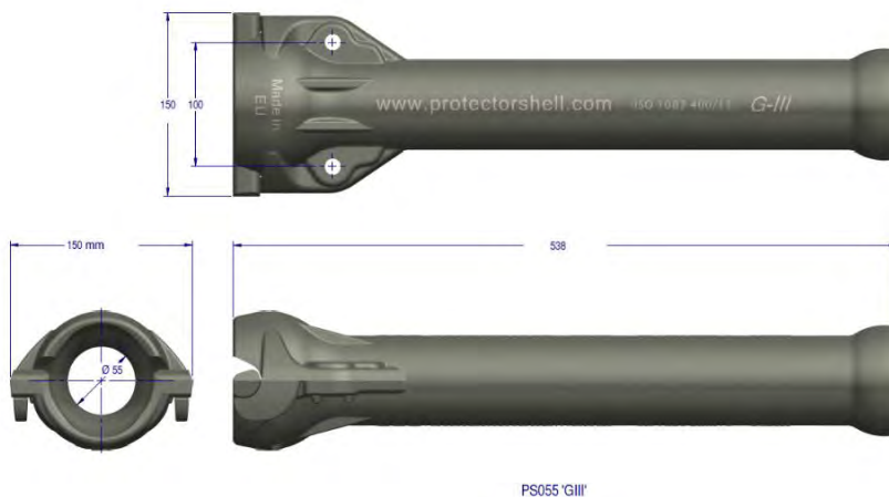
Figure 2-24 Example of Articulated Pipe
