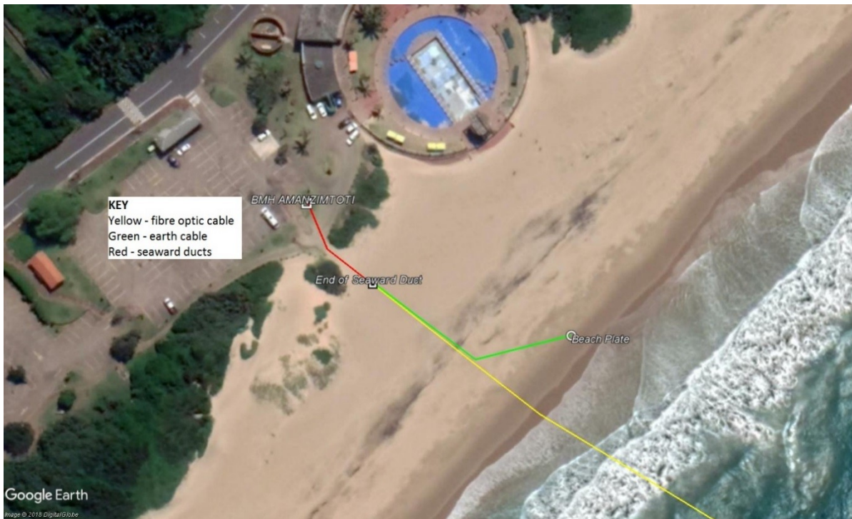
Figure 2-8 Possible Beach Plate Location
