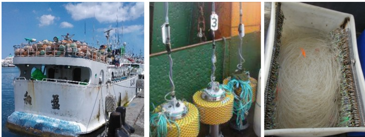
Figure 6-27 Photographs Showing Marker Buoys (left), Radio Buoys (centre) and Monofilament Branch Lines (right)
