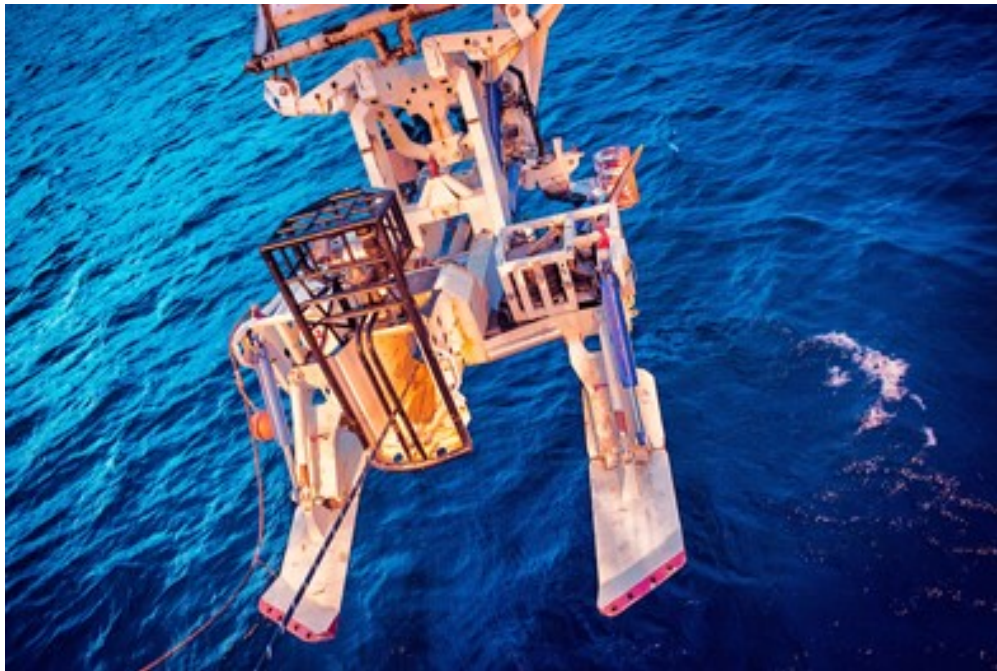
Figure 2-12 Elettra – Taurus2 SMD Plough System
