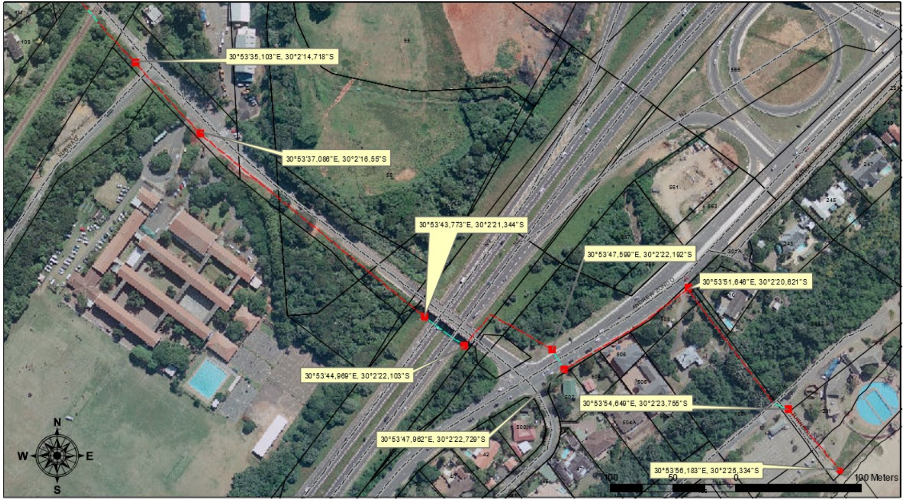
Figure 3-2 Terrestrial Cable Route 1
