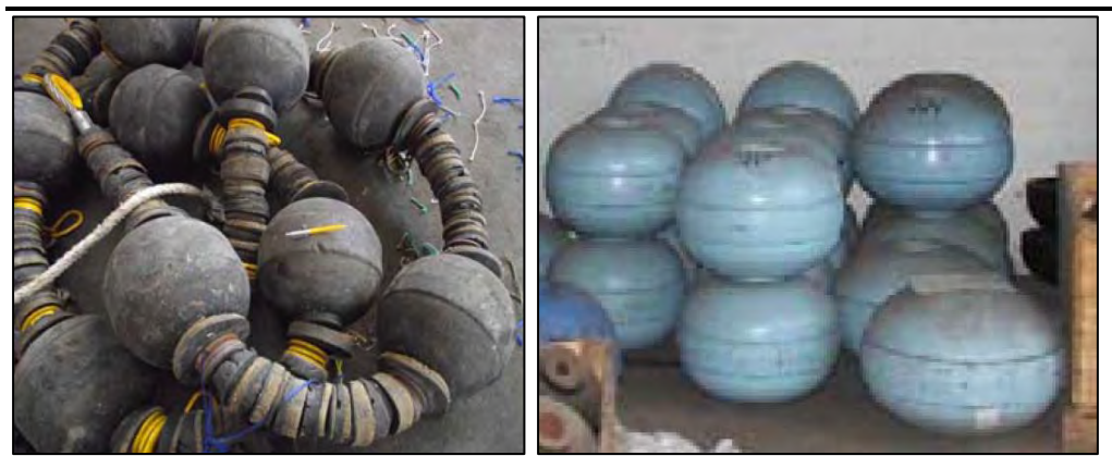
Figure 9.5 Photographs of solid rubber (left) and steel (right) bobbins typically used as part of ground gear in the South African demersal trawl fleet.
