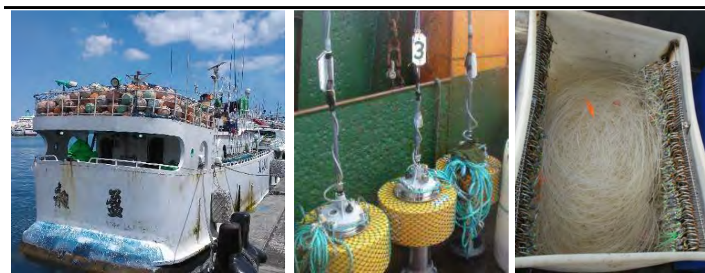
Figure 5.10 Photographs showing marker buoys (left), radio buoys (centre) and monofilament branch lines (right)
