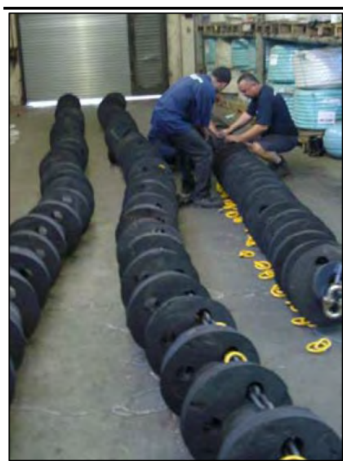
Figure 9.6 Photographs of a footrope with large diameter rubber discs comprising “rockhopper gear” typically used as part of ground gear in the South African demersal trawl fleet.
