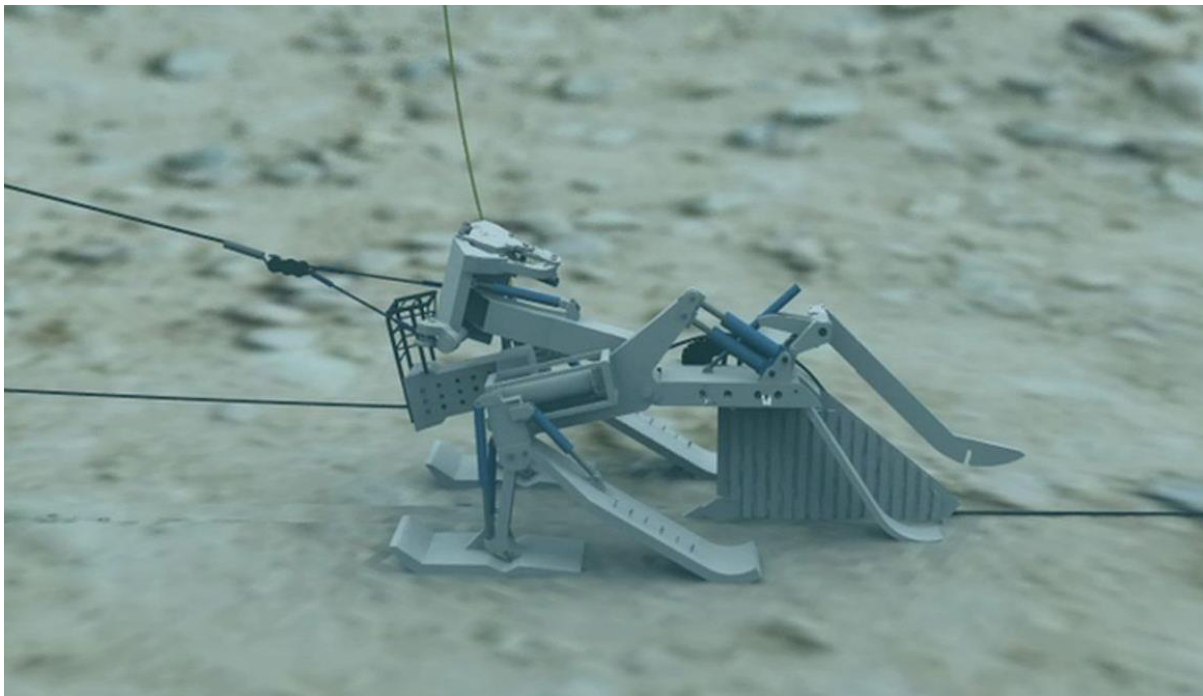
Figure 2-19 Animation of Cable Burial Plough on Seabed
