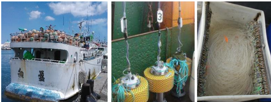
Figure 6-32 Photographs Showing Marker Buoys (left), Radio Buoys (centre) and Monofilament Branch Lines (right)
