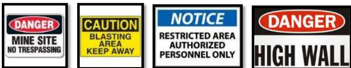
Figure 32: Typical mine fence signage
